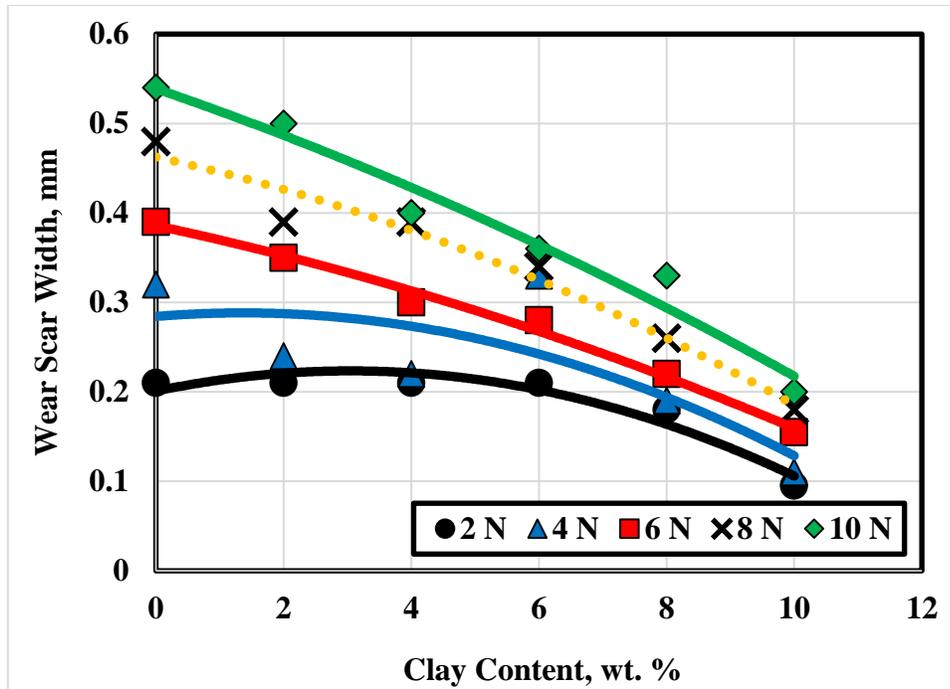
Fig. 11 Effect of clay particles dispersed in the grease blended by 10.0 wt. % oil on wear.
