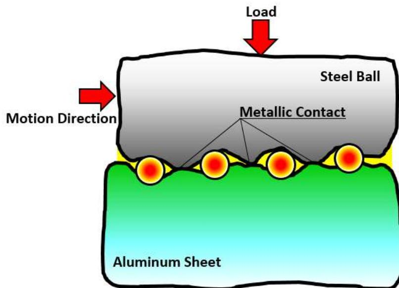
Fig. 4 Illustration of contact in presence of grease dispersed by clay particles.
