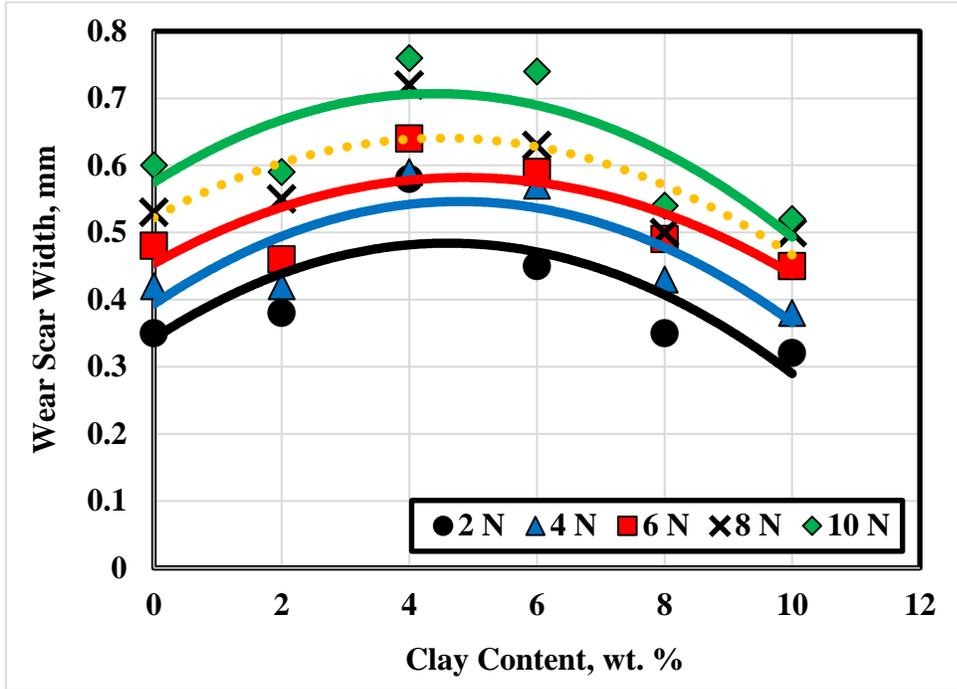
Fig. 9 Effect of clay particles dispersed in the grease on wear.
