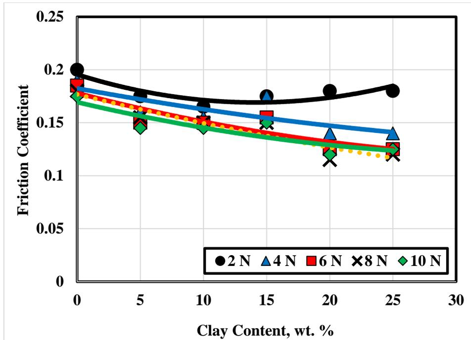
Fig. 7 Effect of clay particles dispersed in the grease blended by 10 wt. % oil on friction coefficient.
