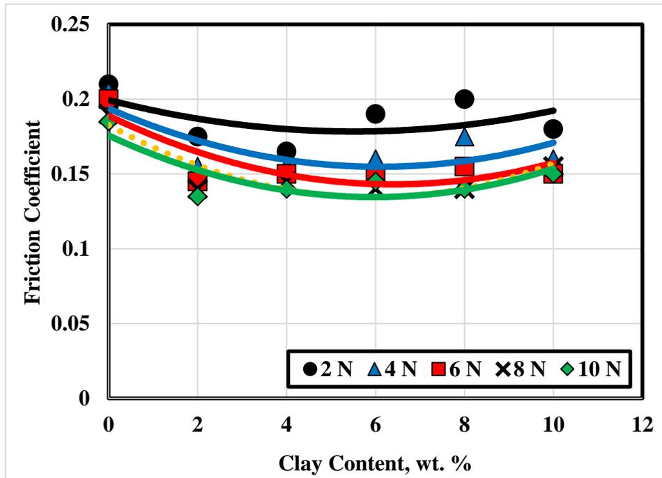
Fig. 6 Effect of clay particles dispersed in the grease blended by 5.0 wt. % oil on friction coefficient.
