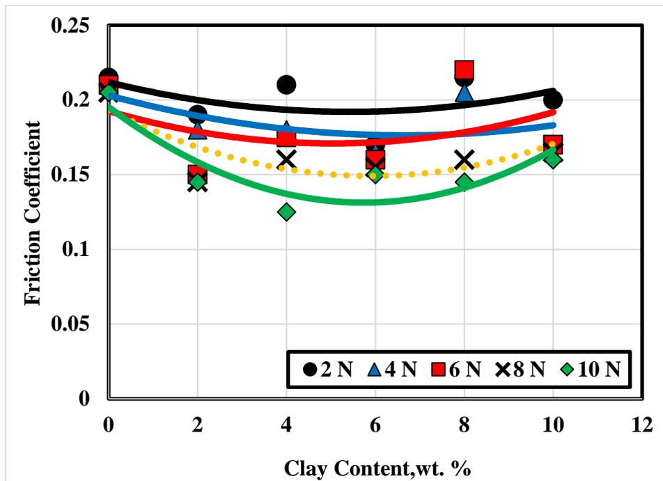
Fig. 2 Effect of clay particles dispersed in the grease on friction coefficient.
