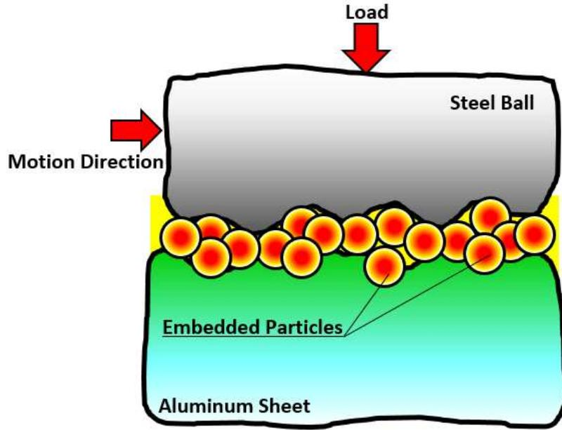
Fig. 5 Illustration of the contact in presence of grease dispersed by relatively higher clay content.
