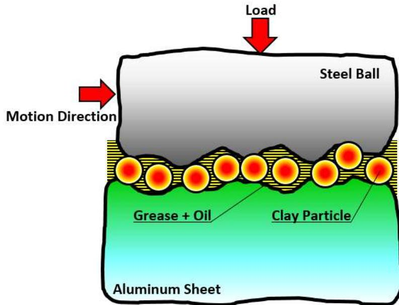
Fig. 8 Illustration of the contact in presence of grease blended by paraffin oil and dispersed by clay content.
