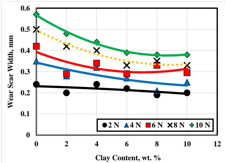
Fig. 10 Effect of clay particles dispersed in the grease blended by 5.0 wt. % oil on wear.
