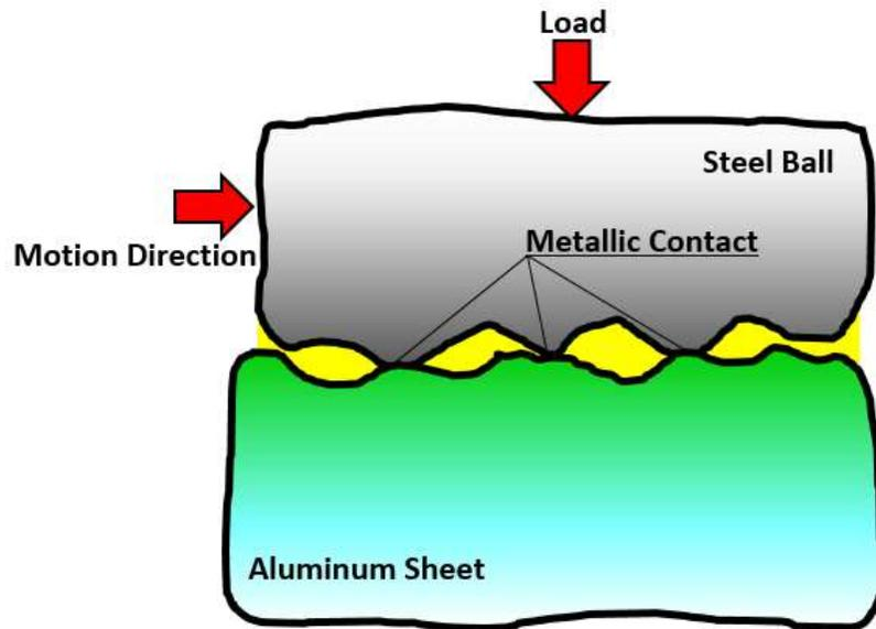
Fig. 3 Metallic contact of the sliding surfaces in the presence of grease free of clay particles.
