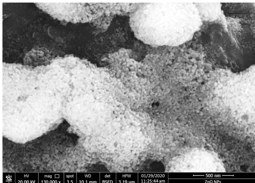
**Fig. 1. SEM for Zn oxide nanoparticles**
