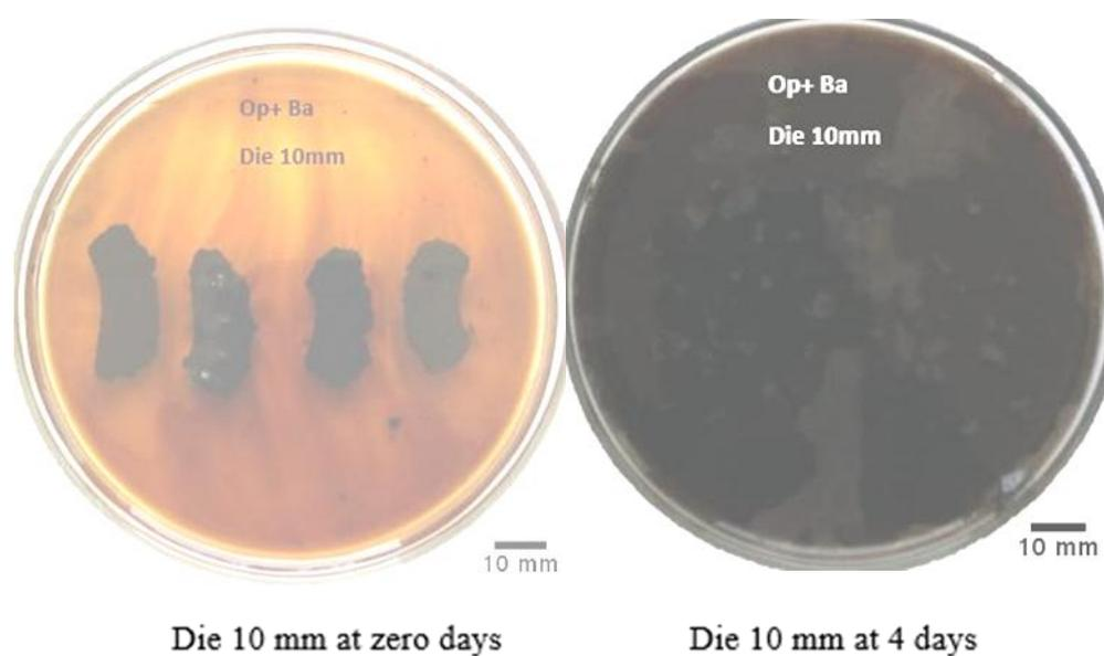
**Fig. 7. Degradation of pellets manufactured using die 10 mm. This image is for demonstrates the instability of pellets at die 10 mm.**
