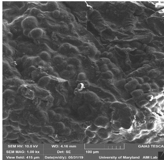
**Fig. 3. SEM images of olive pomace pellets at 5000X magnification from outer sphere**
