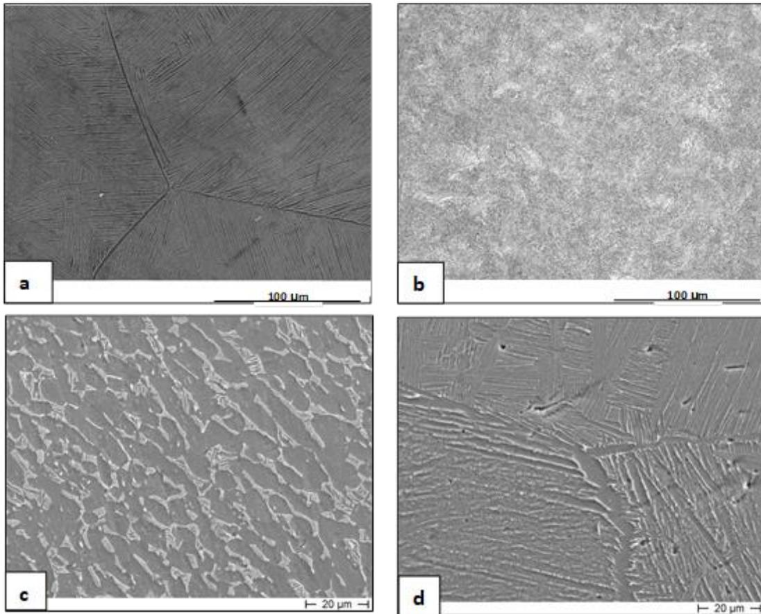
**Fig. 1** Microstructure of the investigated Ti-6Al-4V alloy under different conditions (a- As-cast, b- Swaged, c- ST+A at 850 °C, d- ST+A at 1050 °C).
