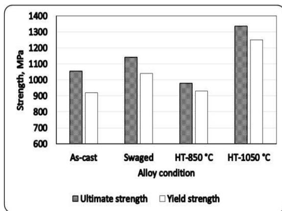
**Fig. 3** The correlation between the investigated Ti-6Al4V alloy condition and strength.
