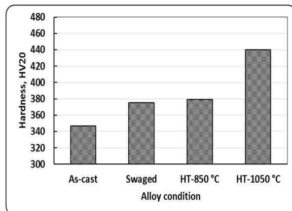
**Fig. 2** The correlation between the investigated Ti-6Al4V alloy condition and hardness.
