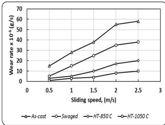
**Fig. 4** Wear rat of the studied Ti-6Al-4V alloy as a function of sliding speed.
