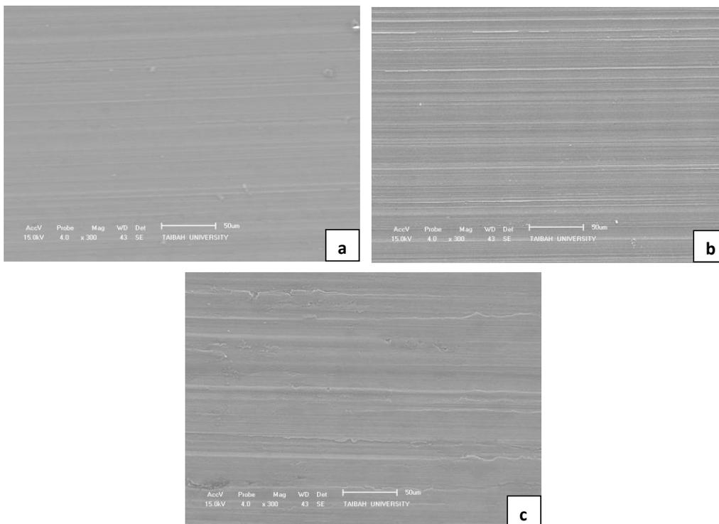
**Fig. 5** SEM images of the wear track surfaces on Ti-6Al-4V samples at different sliding speeds: a- 0.5 m/s, b- 1.5 m/s, and c- 2 m/s.
