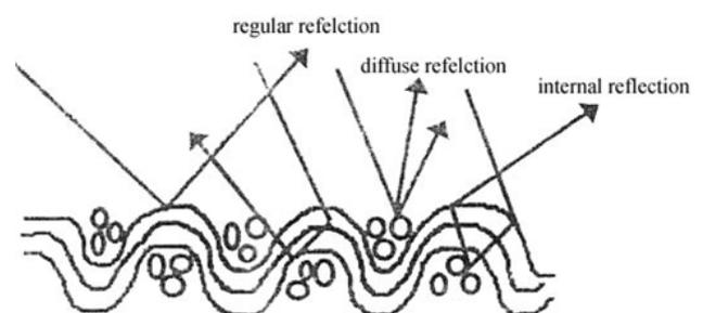
Fig .1 Schematic diagram light reflection from surface of textile.
