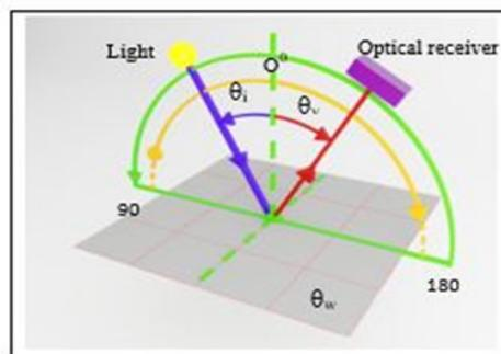
Fig.3. The Measuring geometry, Illumination angle ( $\theta_i$ ), Viewing angle ( $\theta_v$ ) and Rotating angle ( $\theta_w$ ).
