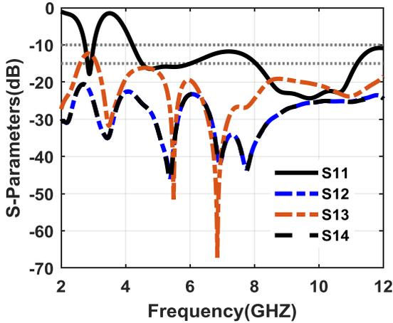
Fig.7: Simulated S-parameters of the MIMO antenna.
