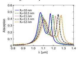
Figure.2. Absorption spectra of the model with various nanoparticle semi-minor axes
