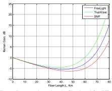
Fig. 6 a Raman gain against the fiber lengthfor different fiber types at 800mW pump power according to basic model.
