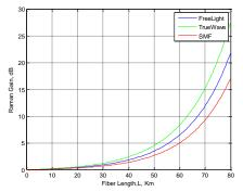
Fig. 6 b Raman gain against the fiber length for different fiber types at 800mW pump power according to proposed system.
