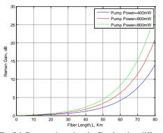
Fig. 5, b Raman gain against the fiber length at different pump powers for Freelight according to proposed system.
