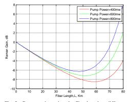
Fig. 3 a Raman gain against the fiber length at different pump powers for SMF according to basic model.
