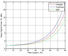
Fig. 7 b Output signal power against fiber length at 800mW pumping power and -5dBm input signal power according to proposed system.
