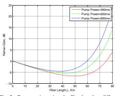
Fig. 5 a Raman gain against the fiber length at different pump powers for Truewave according to basic model.
