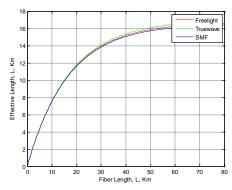
Figure 8 Relation between the Effective Length and Fiber Length for Different Fiber Types
