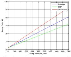
Fig. 2a Raman gain against the pumping power for different fiber types according to basic model.
