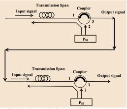
Fig. 2 Design model of two amplifiers are cascaded.
