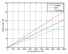
Fig. 2b Raman gain against the pump power for different fiber types according to proposed system.
