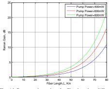
Fig. 4 b Raman gain against the fiber length at different pump powers for Freelight according to proposed system
