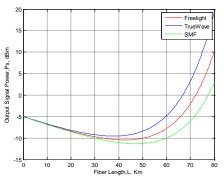
Fig. 7aOutput signal power against fiber length at 800mW pumping power and -5dBm input signal power according to basic model.
