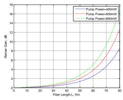
Fig. 3 b Raman gain against the fiber length at different pump powers for SMF according to proposed system.
