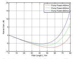
Fig. 4 a Raman gain against the fiber length at different pump powers for Freelight according to basic model.
