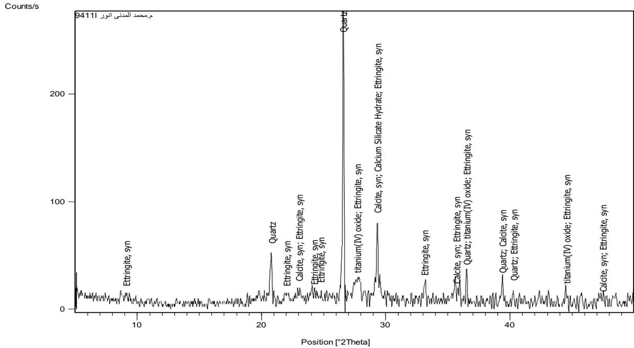
**Fig.7. XRD Pattern of a Specimen after 14 Days**
