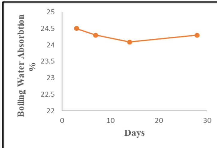
**Fig.12. Effect of Mechanical Mixing on Boiling Water Absorption at 5% Waste Addition**
