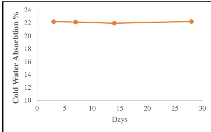
**Fig.11. Effect of Mechanical Mixing on Cold Water Absorption at 5% Waste Addition**
