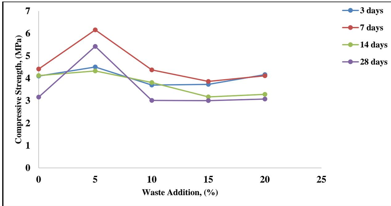
Fig.6. Effect of Waste Addition and Compressive Strength
