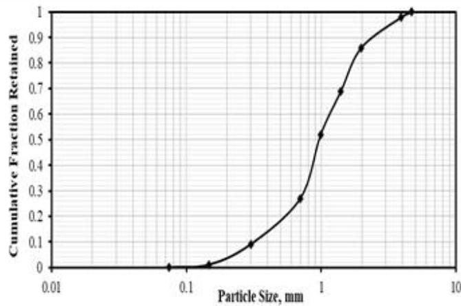
Fig.5. Cumulative Analysis of Dried Milk of Lime
