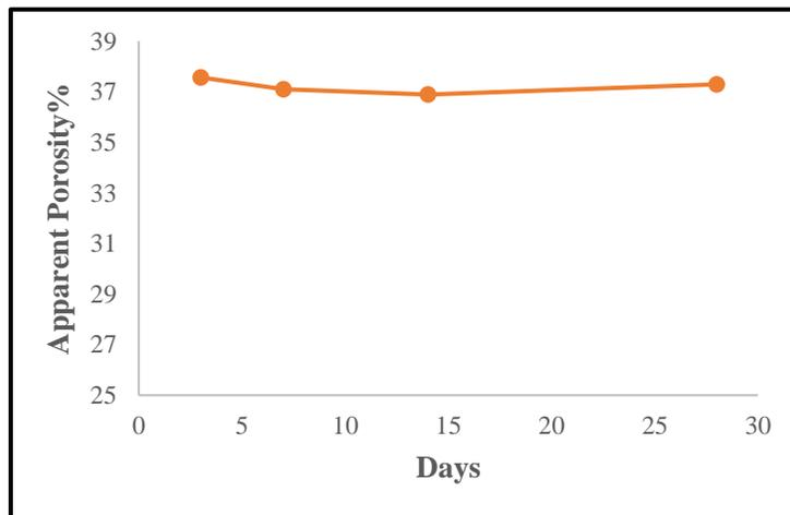
**Fig.10. Effect of Mechanical Mixing on Apparent Porosity at 5% Waste Addition**
