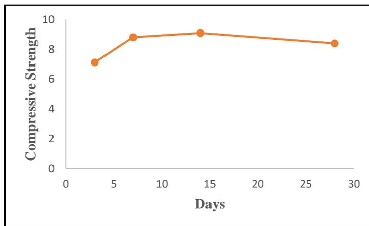
**Fig.8. Effect of Mechanical Mixing on Compressive Strength at 5% Waste Addition**
