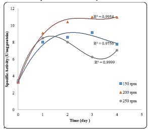
Fig. 8 Comparison between specific activities of amylase produced using three agitation levels for the production of α-amylase
