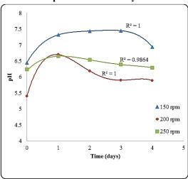
Fig. 10 Comparison between pH recorded of amylase produced using three agitation levels for the production of α-amylase
