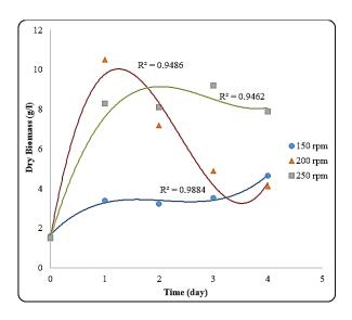
Fig. 6 Comparison between biomass dry weights produced using three agitation levels for the production of α-amylase
