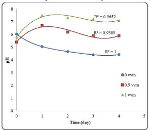
Fig. 5 Comparison between pH recorded for amylase produced using three aeration levels for the production of α-amylase
