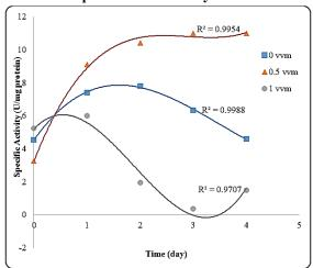
Fig. 3 Comparison between specific activities of amylase produced using three aeration levels for the production of α-amylase
