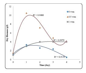
Fig. 1 Comparison between biomass dry weights produced using three aeration levels for the production of α-amylase
