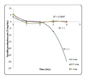
Fig. 4 Comparison between specific production rates of amylase produced using three aeration levels for the production of α-amylase
