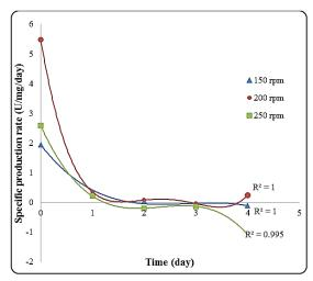
Fig. 9 Comparison between specific production rates of amylase produced using three agitation levels for the production of α-amylase
