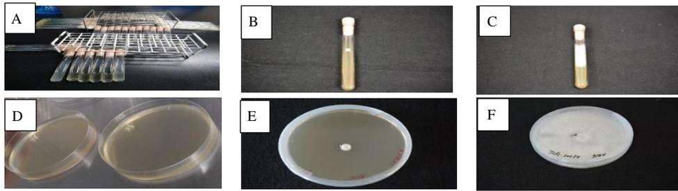
**Figure 1.** Subculturing; **A:** 2% MEA slants preparation, **B:** mycelium inoculation into slants, **C:** Full mycelial growth after 7 days incubation, **D:** 2% MEA Petri-plates preparation, **E:** mycelial disks inoculation from previously prepared slants into plates, **F:** Full mycelial growth after 7 days incubation.
