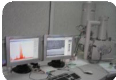
**Figure 2** Quanta Environmental Scanning Electron Microscope (QESEM) computer software.
