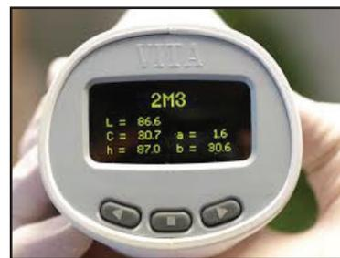
**Fig 6.** The analysis displayed on the spectrophotometer screen giving the components of color L\* a\* b\*.
