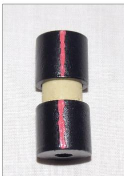
**Fig 4.** The placement of the specimen in the metallic mold.
