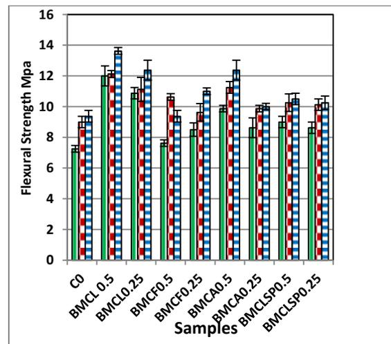
Figure (4): Development of Flexural Strength for All Bacterial and Control Concrete mixes.
