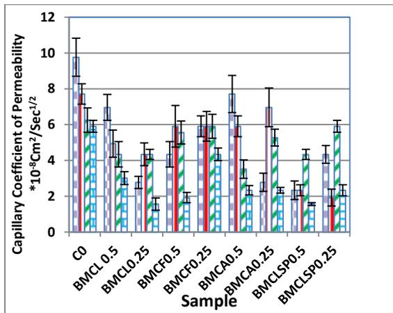
Figure (2): Capillary Permeability Coefficient (K) for Bacterial and Control Concrete after 24hours.
