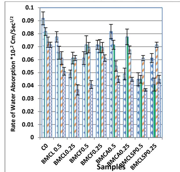
Figure (1): Rate of Water Absorption for Bacterial and Control Concrete after 24 hours.
