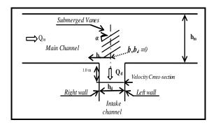
Fig. 4 Layout of the vanes
