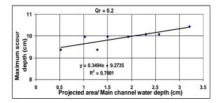
Fig. 14 Regression curve for maximum scour depth prediction  $(b_v/b_d = 0.5, Q_r = 0.2)$
