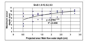
Fig. 16 Regression curve for maximum scour depth prediction ( $b_v/b_d = 0.5$ ,  $Q_r = 0.1$ , 0.15, 02, 0.3)
