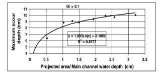
Fig. 12 Regression curve for maximum scour depth prediction ( $b_v/b_d = 0.5$ ,  $Q_r = 0.1$ )
