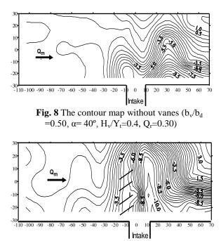
Fig. 9 The contour map using single row of vanes  $(b_v/b_d = 0.50, \alpha = 40^\circ, H_v/Y_t = 0.4, Q_r = 0.30)$
