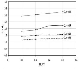
Fig.7 Relationship between  $d_s/d_{sw}$  and  $H_v/Y_t$ , for different  $Q_r$
