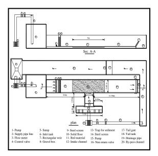
Fig. 3 Flume layout
