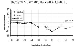
Fig. 11 Scour hole profile using single row of vanes  $(b_v/b_d = 0.50, \alpha = 40^\circ, H_v/Y_t = 0.4, Q_t = 0.30)$
