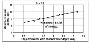
Fig. 15 Regression curve for maximum scour depth prediction ( $b_v/b_d = 0.5$ ,  $Q_r = 0.3$ )
