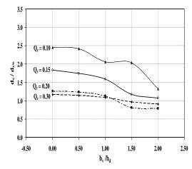
Fig. 5 Relationship between ds/dsw and bv/bd, for different Qr
