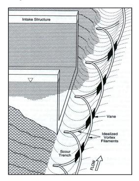
Fig. 2 Conceptual flow pattern and scour trench due to submerged vane (After Brian. D. Barkdool, 1999)
