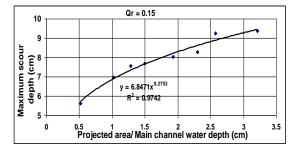
Fig. 13 Regression curve for maximum scour depth prediction ( $b_v/b_d = 0.5$ ,  $Q_r = 0.15$ )
