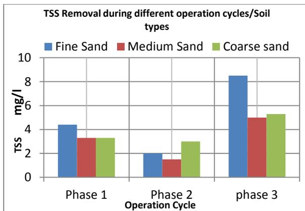
Figure 4. TSS Removal during different operation cycles/Soil types
