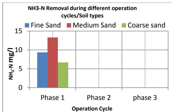
Figure 6. Ammonia Removal during different operation cycles/Soil types
