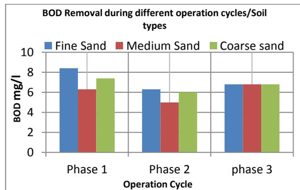
Figure 2. BOD Removal during different operation cycles/Soil types
