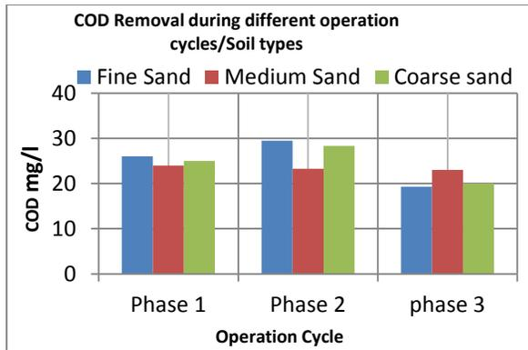
Figure 3. COD Removal during different operation cycles/Soil types
