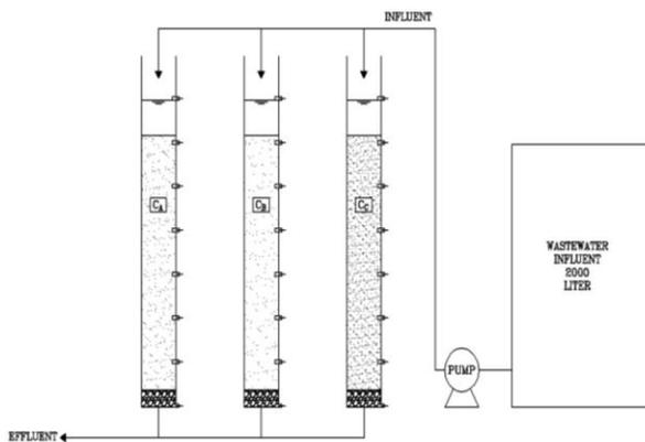
Figure 1. A schematic diagram of the SAT pilot plant system set-up used in this study.
