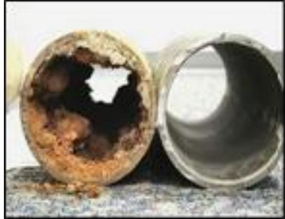
Fig 12: sediments in pipes
