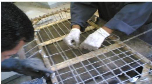
Fig.7: Intertwined GFRP roving submerged in epoxy
