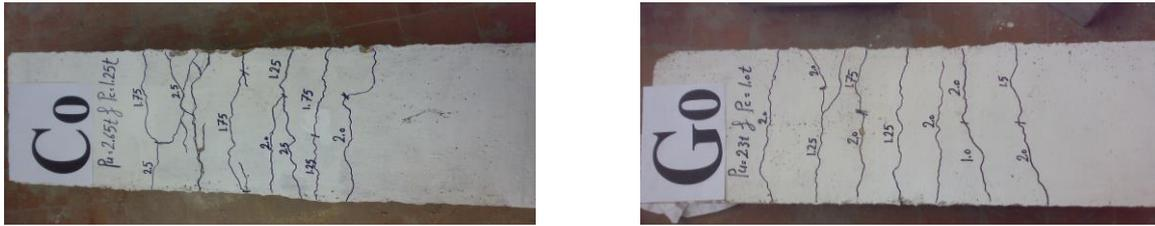
Fig.16: Crack patterns for control slabs (Group 1)
