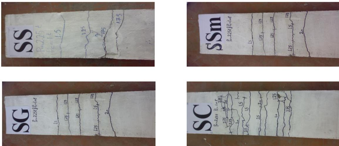
Fig.18: Crack patterns for strengthened slabs (Group 3)
