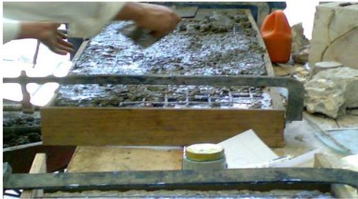
Fig.9: Casting concrete for strengthening layer
