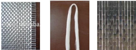
(a) GFRP woven roving wraps (b) E-Glass-roving (c) Sika Wrap Hex -230C
