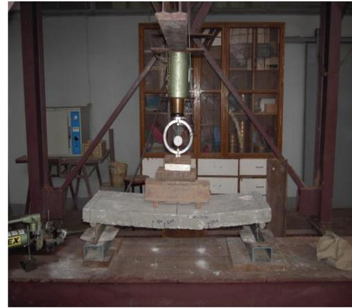
Fig. 4: Control slab S0 during test
