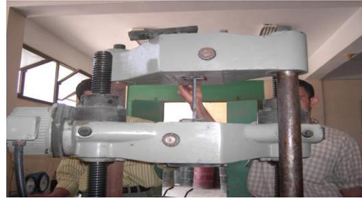
Fig. 10: Testing intertwined GFRP rods
