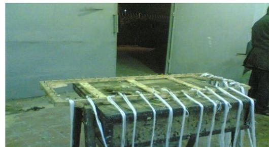
Fig.6: Fixing GFRP roving in nails on loom
