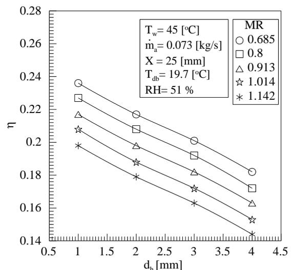
Fig. (9). Effect of injection holes diameter on the cooling tower efficiency for different mass flow rate ratio.
