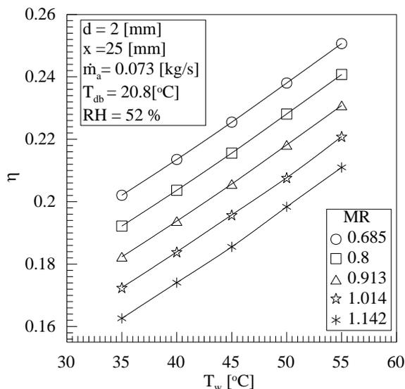
Fig. (2). Effect of water inlet temperature on the effectiveness for different mass flow rate ratio.
