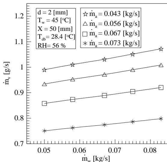
Fig. (8). Effect of water mass flow rate on the vaporization for different air mass flow rate.
