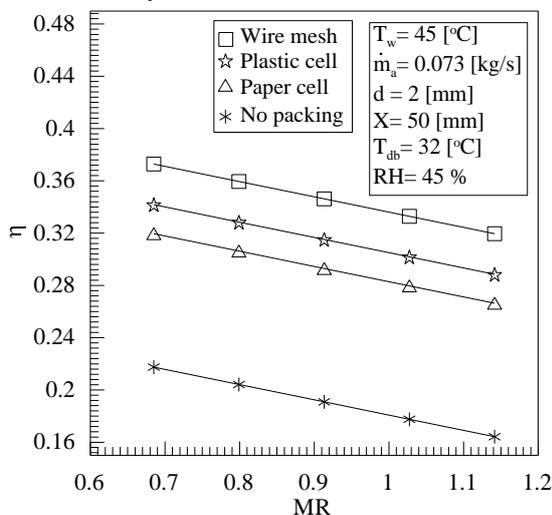
Fig. (15). Cooling tower efficiency versus water/air mass flow ratio (MR) with and without packing
