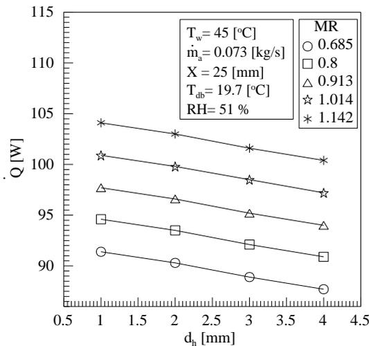
Fig. (10). effect of injection holes diameter on the heat rejected for different mass flow rate ratio.
