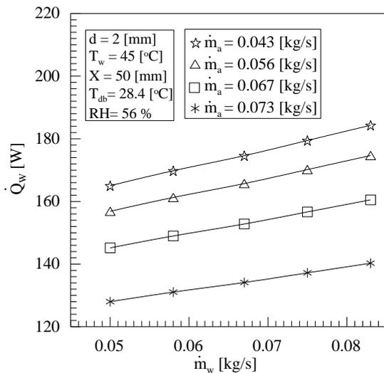
Fig. (7). Effect of water mass flow rate on the heat rejected for different air mass flow rate.
