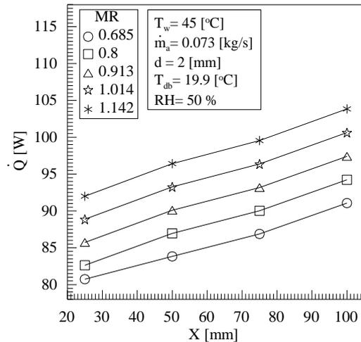
Fig. (13). Effect of interval distance between injection holes on the rejected heat for different mass flow rate ratio.
