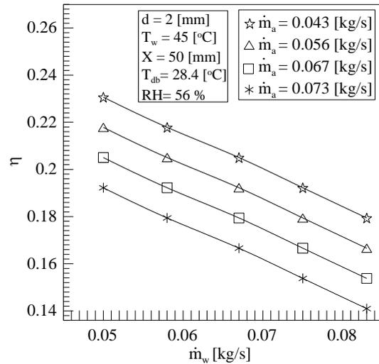
Fig. (6). Effect of water mass flow rate on the cooling tower efficiency for different air mass flow rate.
