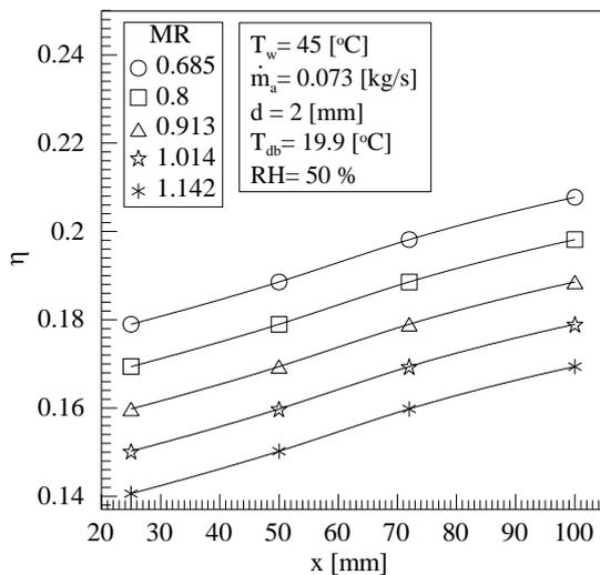
Fig. (12). Effect of interval distance between injection holes on the cooling tower efficiency for different mass flow rate ratio.
