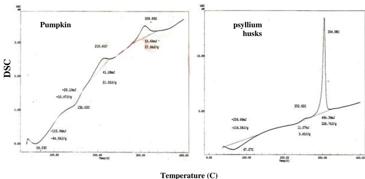
**Fig.(3):** The DSC thermograph of thermal properties of pumpkin and psyllium husks powders.
