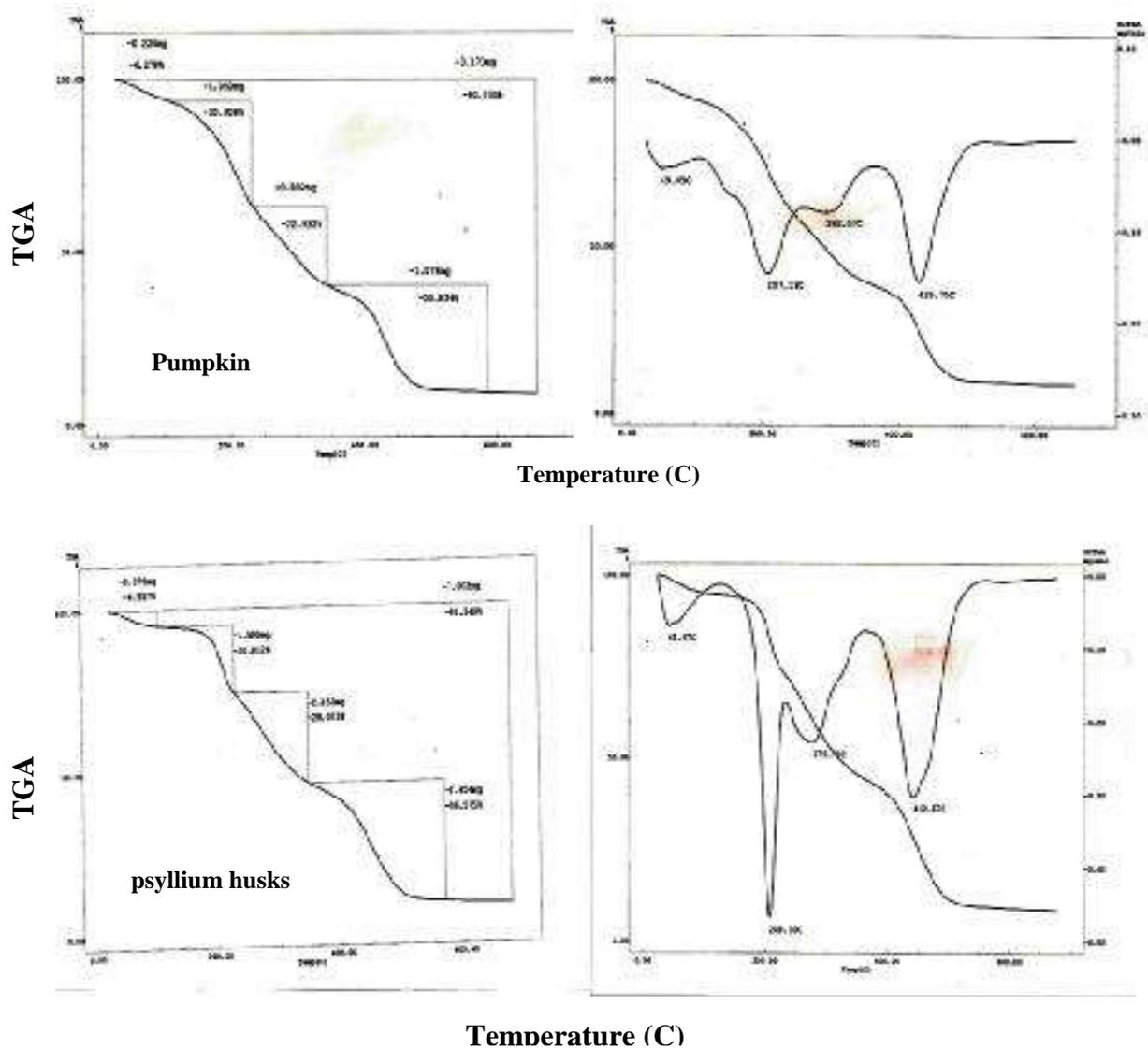
Fig.( 4):Thermogravimetry analysis properties of pumpkin and psyllium husks powders.
