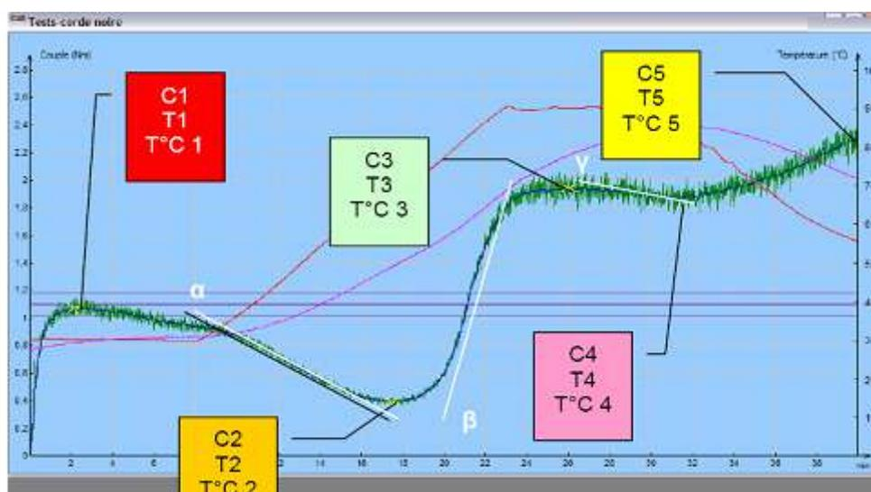
**Fig. (1): Main changes that occur during Mixolab test (after Dubat *et al.*, 2013). Numbers indicate the different areas detected in the curve according to the wheat bread dough changes . (1) Dough development. (2) Protein reduction during heating. (3) Starch gelatinization . (4) Amylase activity . (5) Starch gelling due to cooling .**
