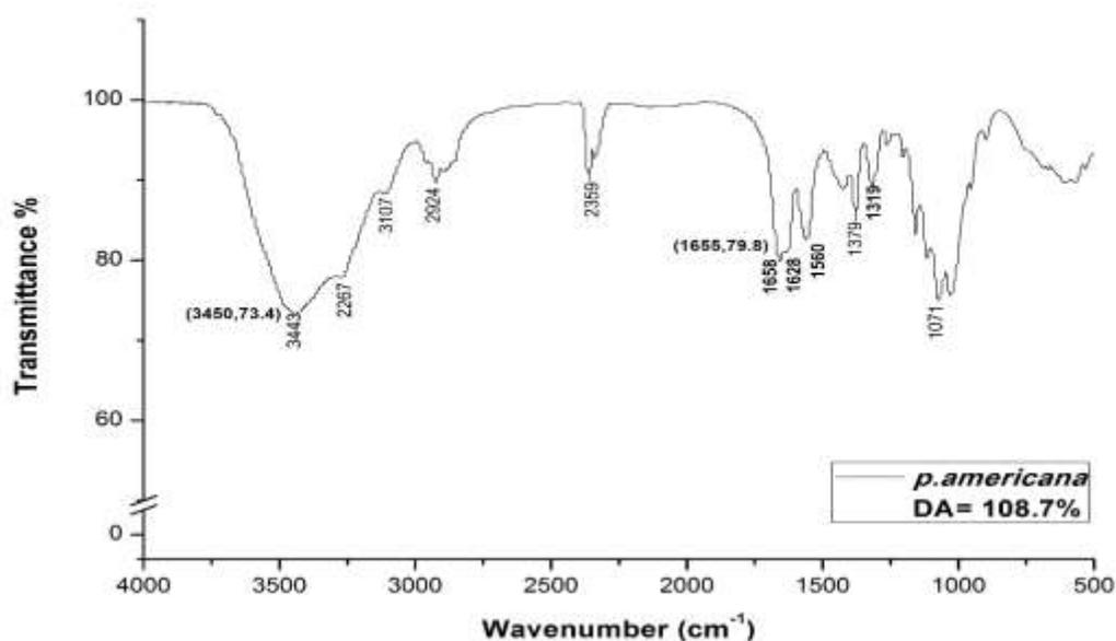
Fig. 1: The IR spectra of the chitin extracted from the American cockroach *P. americana*.
