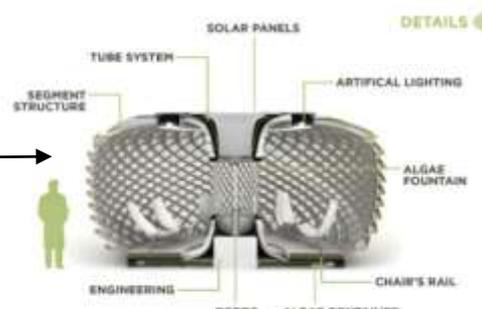
CO<sub>2</sub> and form biomass that is pushed through underground tubes to a nearby filler station. The chamber inside the street lamp is refilled with more algae and water to start the process again (Fig. 10).
