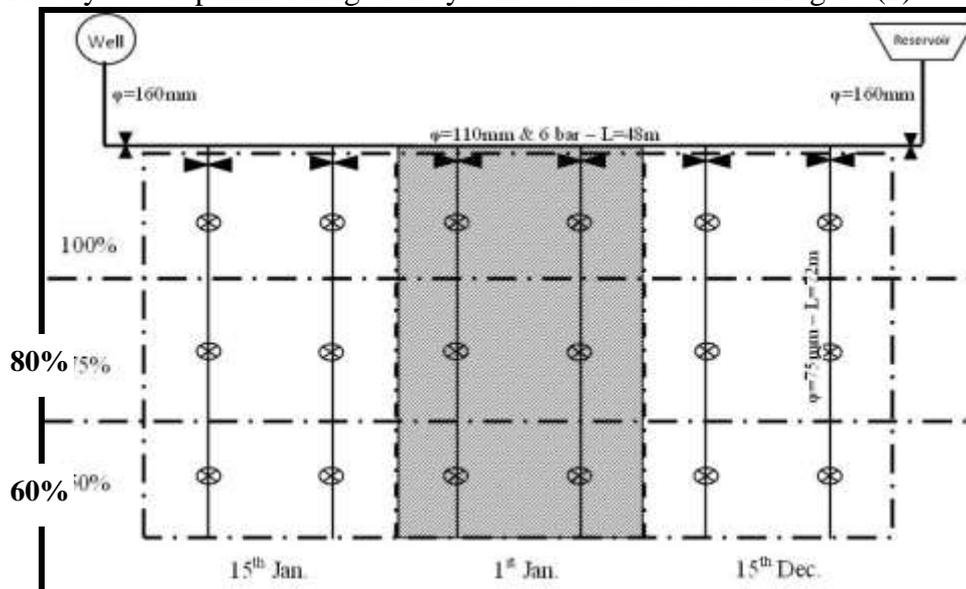
Fig. (2): Layout of sprinkler irrigation system experiments.
