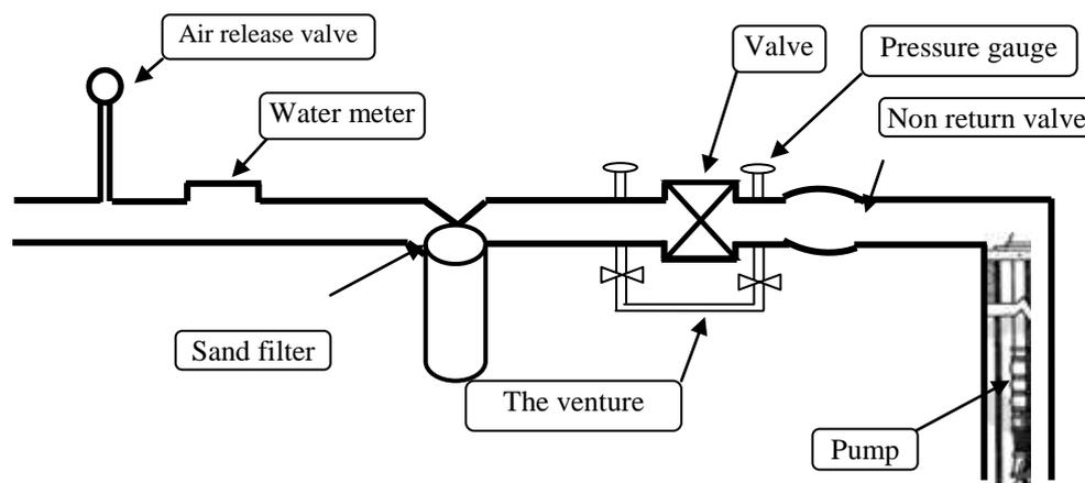
**Fig. (1): The diagram of control unit.**
