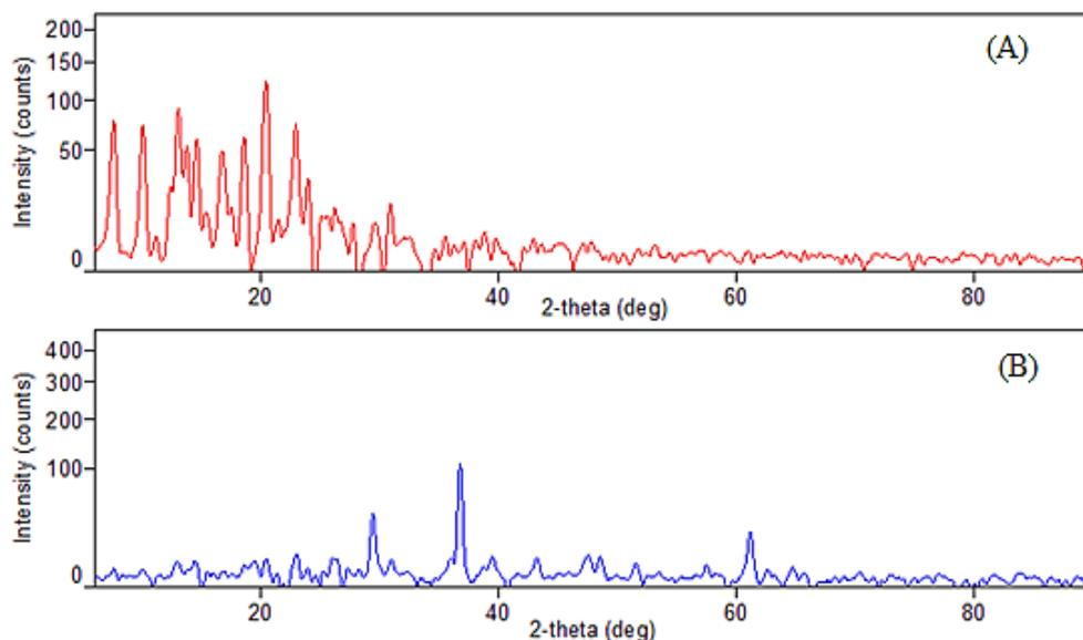
**Fig. 5:** X-ray diffractograms of pure repaglinide (A) and formulation F1 (B).
