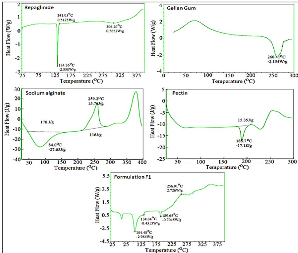
Fig. 6: DSC thermograms of pure repaglinide, sodium alginate, gellan gum, pectin, and formulation F1
