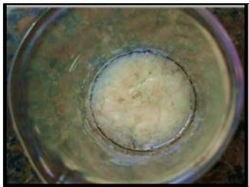
**Fig. 3:** Gel formation of GRFS in presence of 0.1N HCl (pH 1.2).
