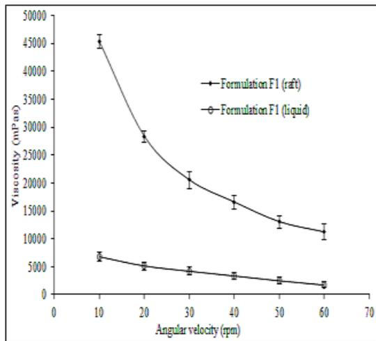
Fig. 7: Viscosity result of formulation F1 (liquid) and formulation F1 (raft) at 10, 20, 30, 40, 50, and 60 rpm (mean ± SD, n= 3).
