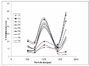
**Fig. 4:** Particle size distribution curves for IBU–GL pellets of different batches.
