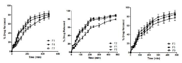
Fig. 6: Effect of amount of GL on the *in-vitro* release of IBU from different prepared batches in phosphate buffer of pH 7.4. Each point is the average of 3 experiments.
