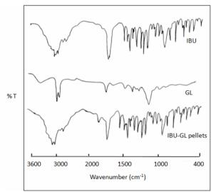
**Fig. 2:** IR spectra of IBU, Gelucire 50/13, and IBU-Gelucire pellets.
