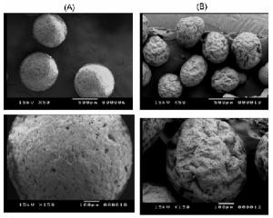
Fig. 1: SEM microphotographs of IBU-GL pellets.(A): Pellets of 10% w/w GL. (B): Pellets of 15% w/w GL.
