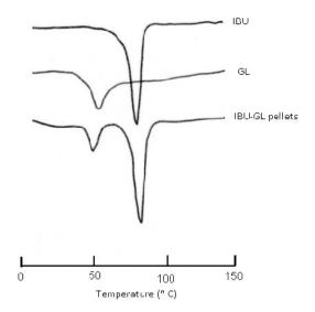
**Fig. 3:** DSC thermograms of IBU, Gelucire 50/13, and IBU-Gelucire pellets.
