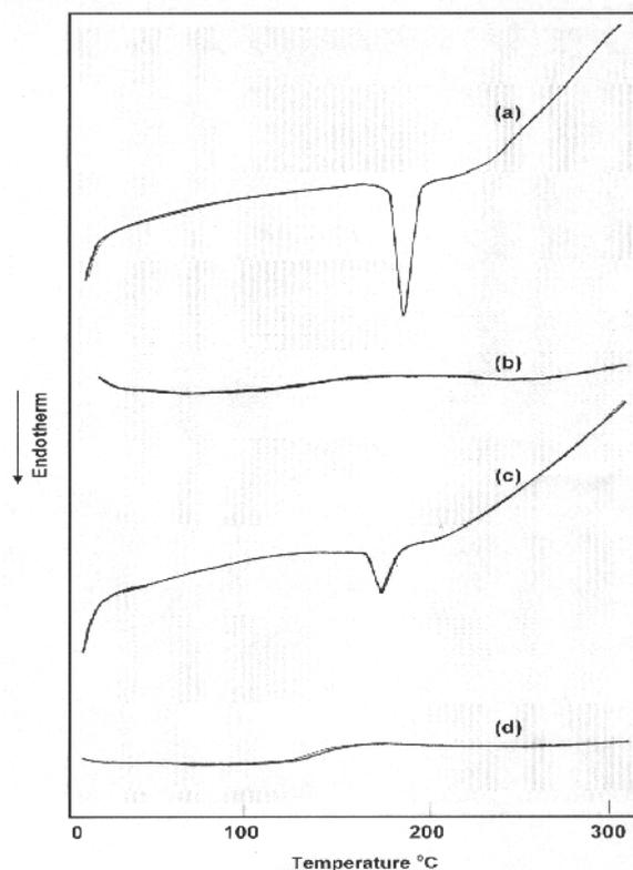
**Fig. 5:** DSC thermograms of **a:** drug alone, **b:** chitosan L\* powder, **c:** physical mixture of Tr.HCl-chitosan L\* and **d:** cast film of Tr.HCl-chitosan L\*.
