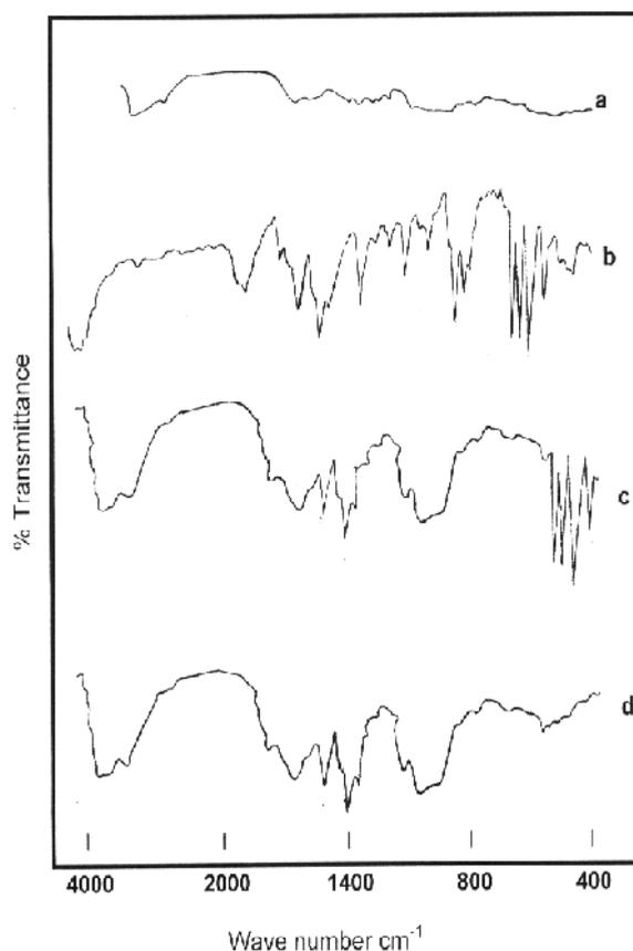
**Fig. 4:** IR spectra of **a:** chitosan L\* powder, **b:** drug alone powder, **c:** physical mixture of Tr.HCl-chitosan L\* and **d:** cast film of Tr.HCl-chitosan L\*.
