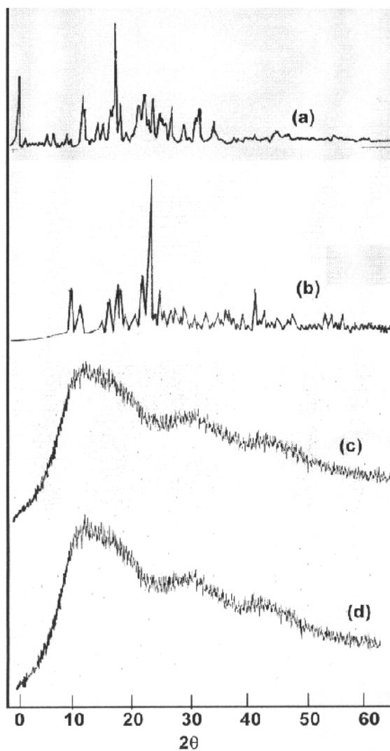
**Fig. 6:** X-ray pattern of **a:** drug alone, **b:** chitosan L\* powder, **c:** physical mixture of Tr.HCl-chitosan L\* and **d:** cast film of Tr.HCl-chitosan L\*.
