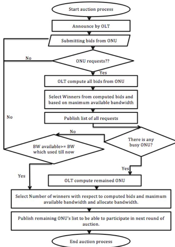
Fig. 3. Schematic diagram of the overall process in the S-MAAT method
