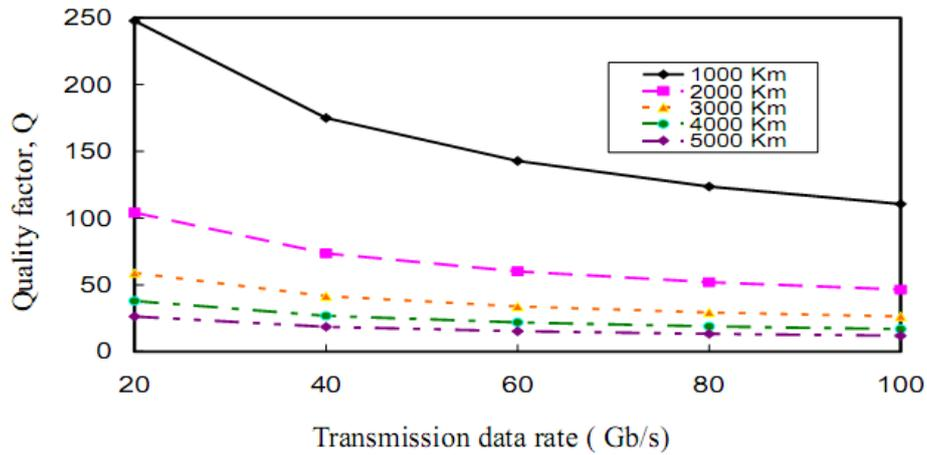
Fig. 7. Signal quality factor in relation to transmission data rate at different values of propagation distance.
