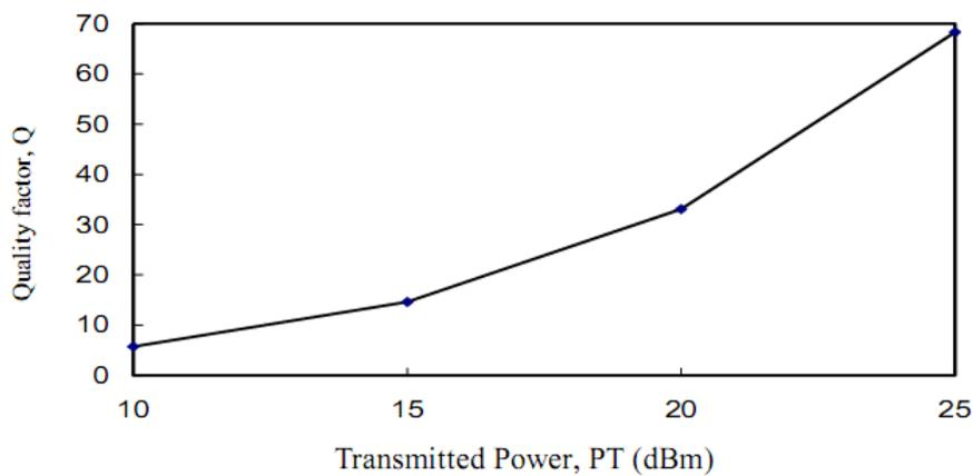
Fig. 8. Signal quality factor in relation transmitted power.
