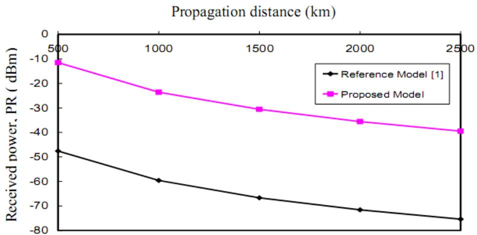
Fig. 2. Received power in relation to propagation distance using reference model [1] and proposed model.
