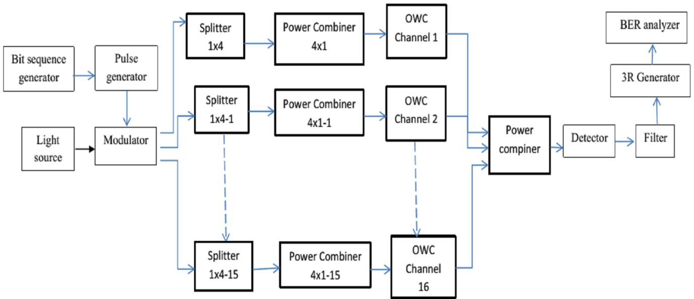
Fig. 1. B. Simulation Model 16 TX/RX IsOWC system.
