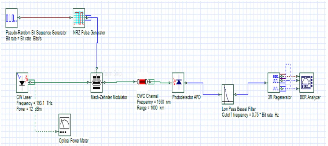
Fig. 1. A. Simple model of IsOWC system.
