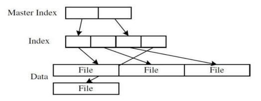
Figure 3: Reading Files from HAR
