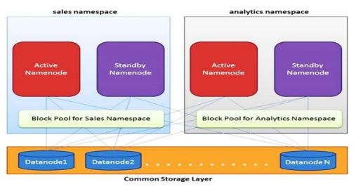
Figure 4: Federated NameNode Architecture
