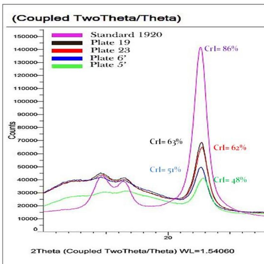
Fig. 6. Shows X-Ray diffraction analysis for determination of paper crystallinity for some historical plates compared to Whatman paper (1920s).
