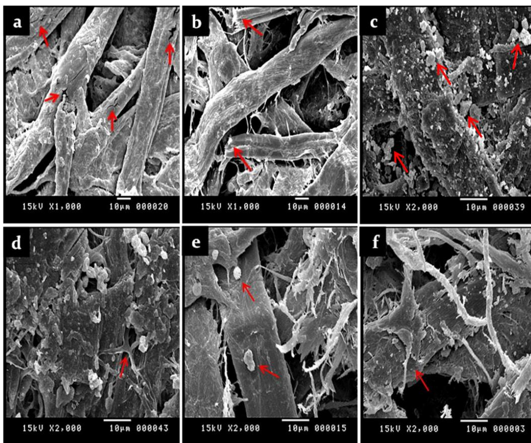
**Fig. 5. SEM images of the historical plates show natural ageing effects on the cellulose fibers, (a) Cracks, (b) broken fibers, (c) Particles cover the surface of the paper fibers, (d, e) Spores and fungal hyphae cover the paper fibers, (f) Erosion on the surface of the fibers as result fungal contamination.**
