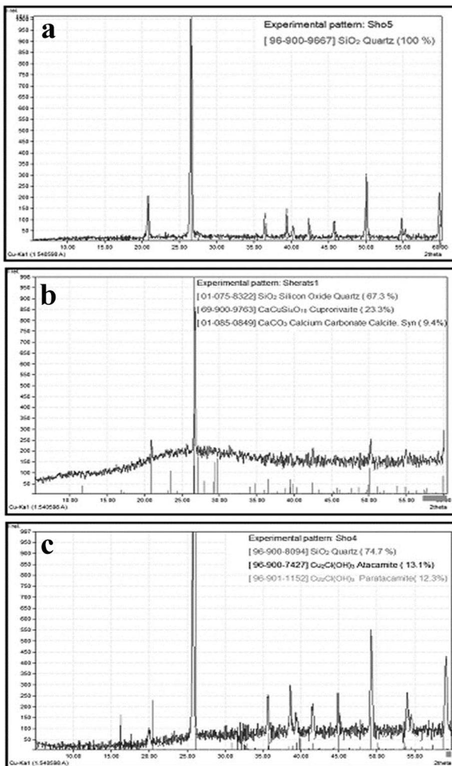
Fig. 7. XRD patterns of faience samples, a. Pattern of the core, b. Pattern of the glaze color, c. Pattern of the glaze discoloration
