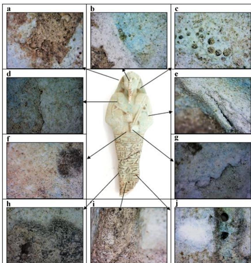
**Fig. 5.** Shows the examination by USB digital light microscope (the front), a. Dirt and dust penetrating the surface, b. Loss of glaze, c. holes in the glaze layer (manufacturing defects), d. Micro-cracks, e. Glaze flaking, f. Black stains in the glaze, g. Detaching and peeling of glaze layer, h and i. Dust and sand inside the hieroglyph's letters, j. Big holes with dirt
