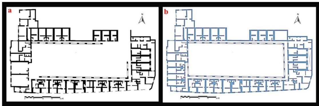
**Fig. 8. The horizontal plan of the first floor (a) The current situation after demolition with the effect of deterioration factors, (b) Proposal after reconstruction work**
