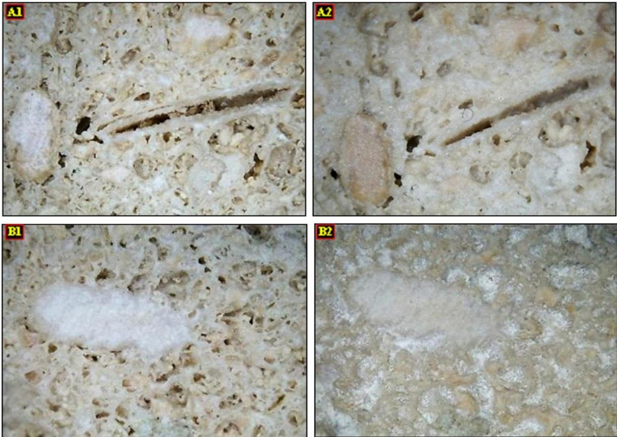
**Fig. 8: Digital Microscope (DM) images of the "Mangabi" stone specimens before and after the consolidation treatment, magnification 100 X: (A1) the stone before the treatment, (A2) the same area after the treatment with Wacker OH-100, (B1) the stone before the treatment, (B2) the same area after the treatment with CaLoSiL.**
