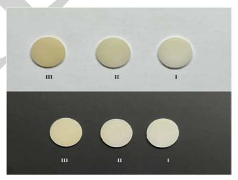
**Figure (2):** Transparency Parameter (TP) at different parts of specimens of different thicknesses tested on white and black paper
