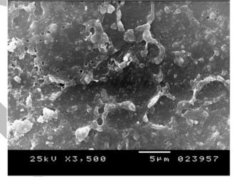
**Fig. (5):** Scanning electron micrograph ( $\times$ 3500) showing the adhesive resin on the enamel surface of the debonded specimen from Group A (antioxidant treatment).
