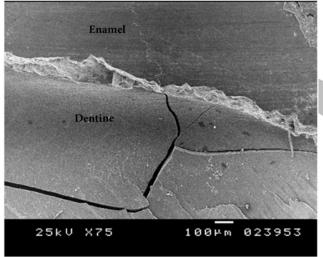
Fig. (3): Scanning electron micrograph ( $\times$ 75) showing cohesive failure pattern on debonded enamel specimen from Group D (control group).
