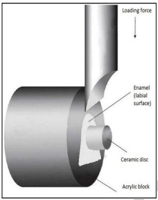
**Fig. (1):** Schematic diagram of shear bond strength testing using universal testing machine.
