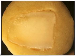
Fig. (4): Adhesive failure in Group A (antioxidant treatment)
