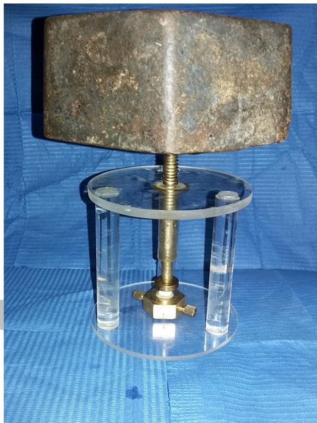
Fig. 4: Custom-made load device.
