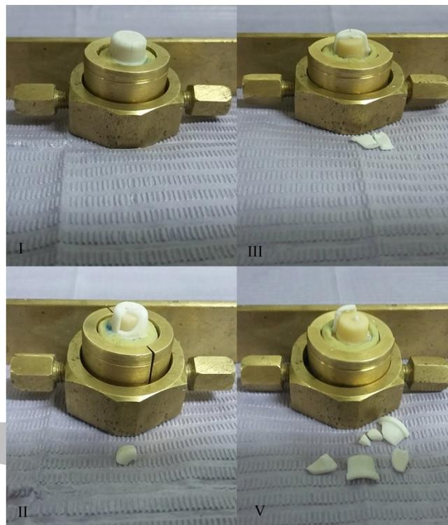
**Fig 7:** Different patterns of crown fracture.
