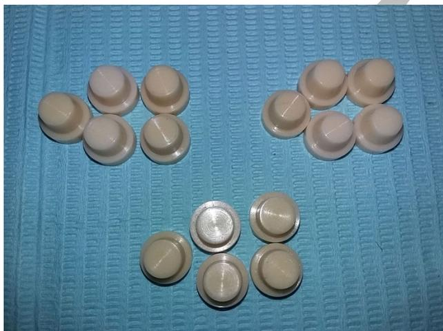
**Fig. 2:** Epoxy resin die.
