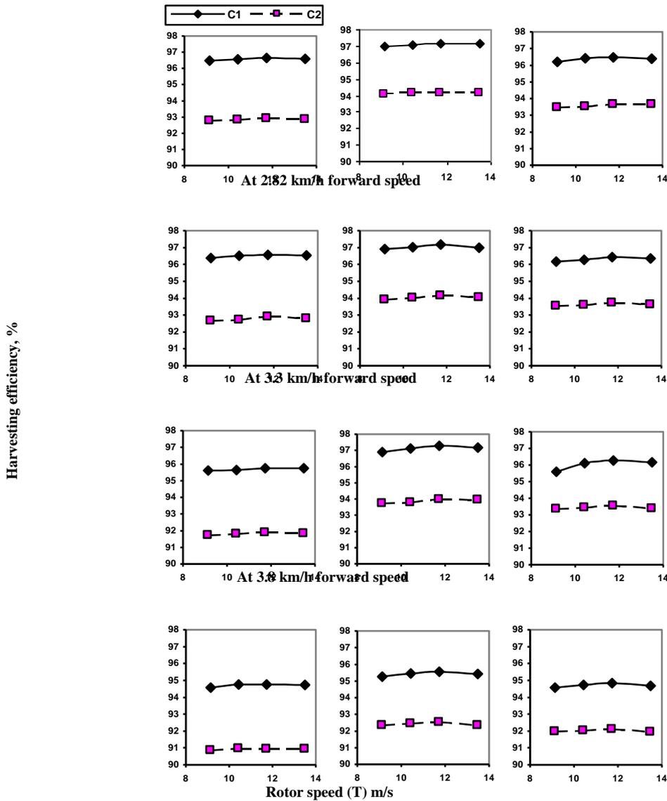
Figure 2. Effect of rotor speed and rotor-concave clearance ratio on harvesting efficiency, at different forward speeds and seed moisture contents ( $c_1 = 1.5$ ,  $c_2=1.3$ ).
