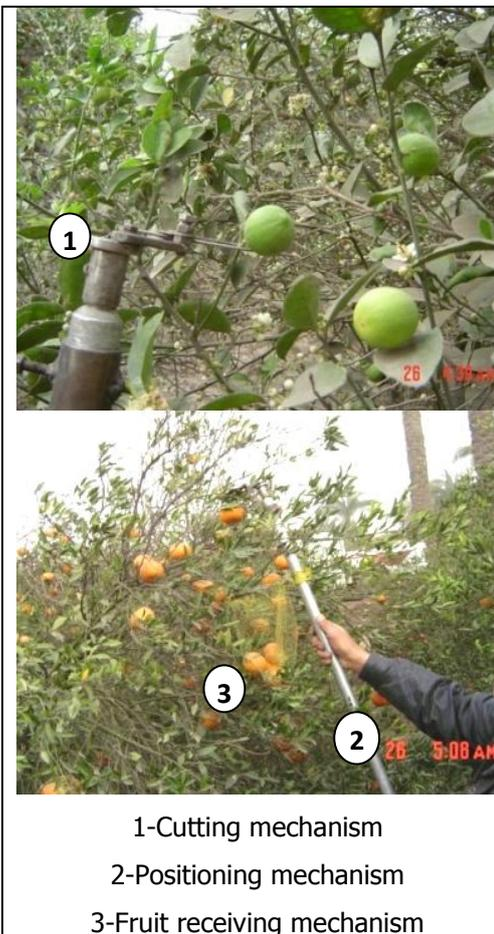
Fig. 3. The main components of electrical scissors head.
