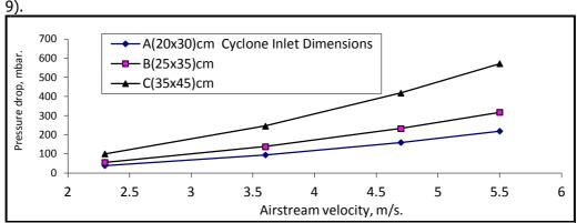
Fig. 8.The pressure drop versus airstream velocity at different cyclone inlet dimensions.
