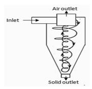
Fig. 1: Schematic presentation of the flow in a 2D2D cyclone before development.
