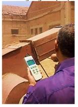
Fig.4: Measuring airstream velocity by the anemometer.
