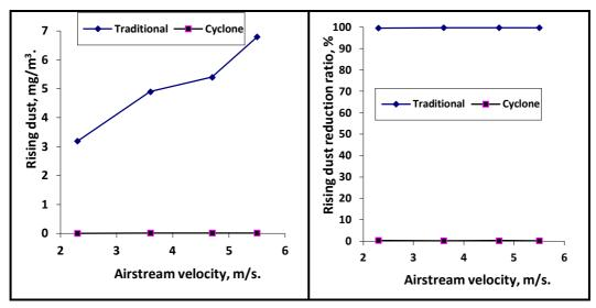
Fig 10. Effect of airstream velocity on rising dust, mg/m³.
