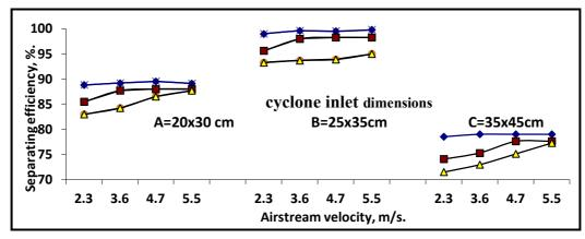
Fig. 6. Effect of airstream velocity, vortex finder length and cyclone inlet dimensions under cyclone outlet ratios of 0.80 on separating efficiency.
