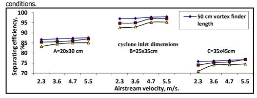
Fig. 5. Effect of airstream velocity, vortex finder length and cyclone inlet dimensions under cyclone outlet ratios of 0.75 on separating efficiency.
