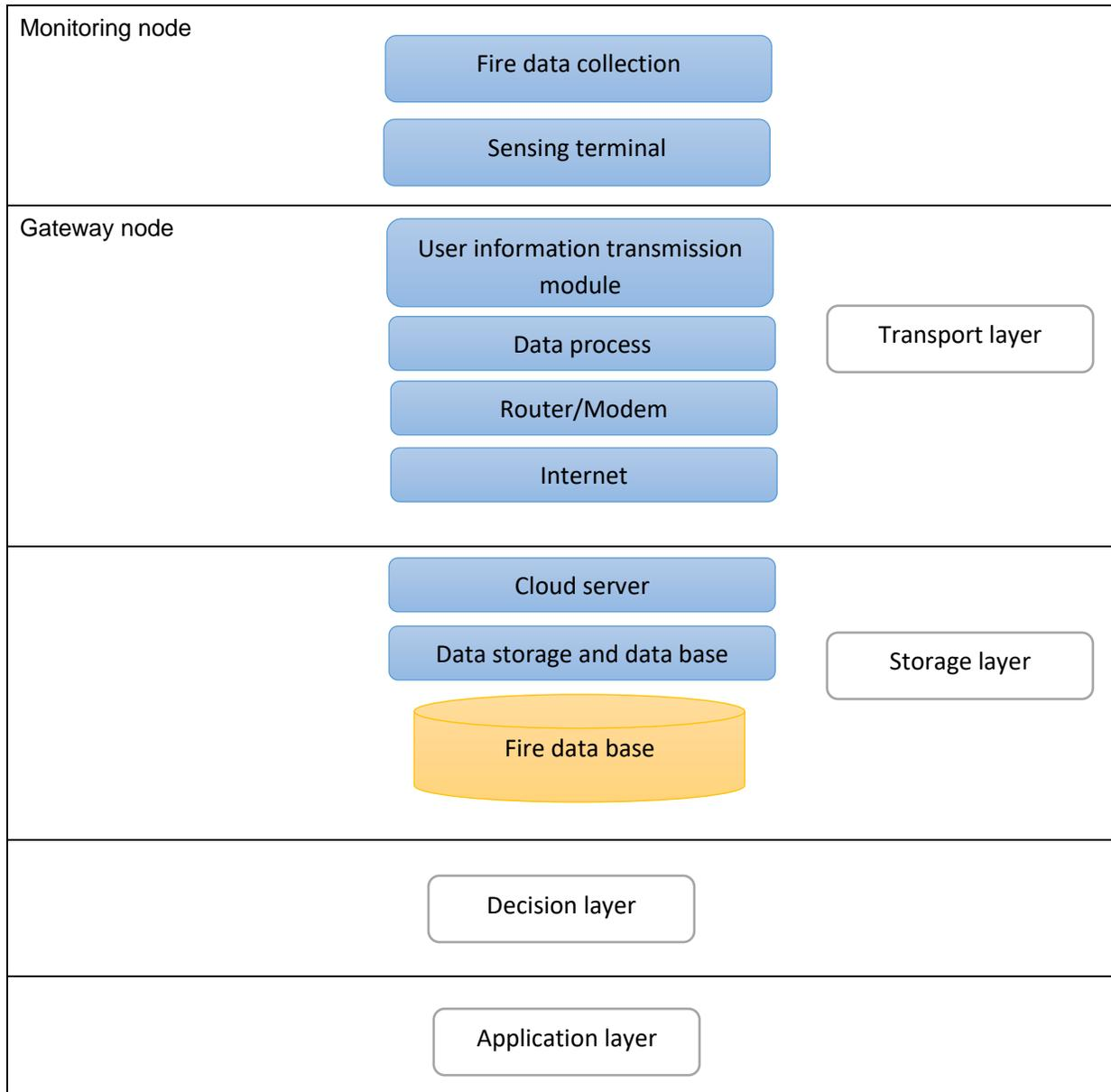
**Figure 2:** The framework of fire monitoring information system
