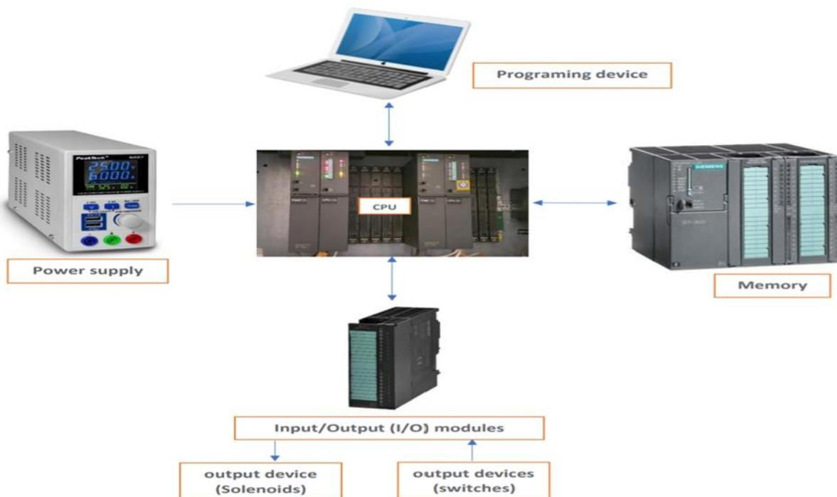
Figure 4: Block diagram of PLC.
