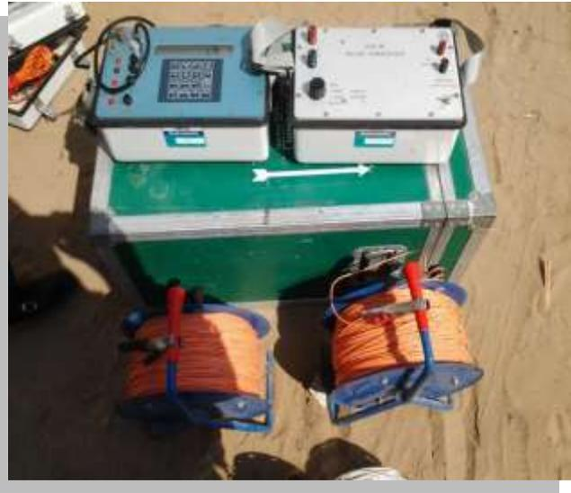
**Fig. 6.** Eleric-T resistivity meter, IRIS Instruments, France
