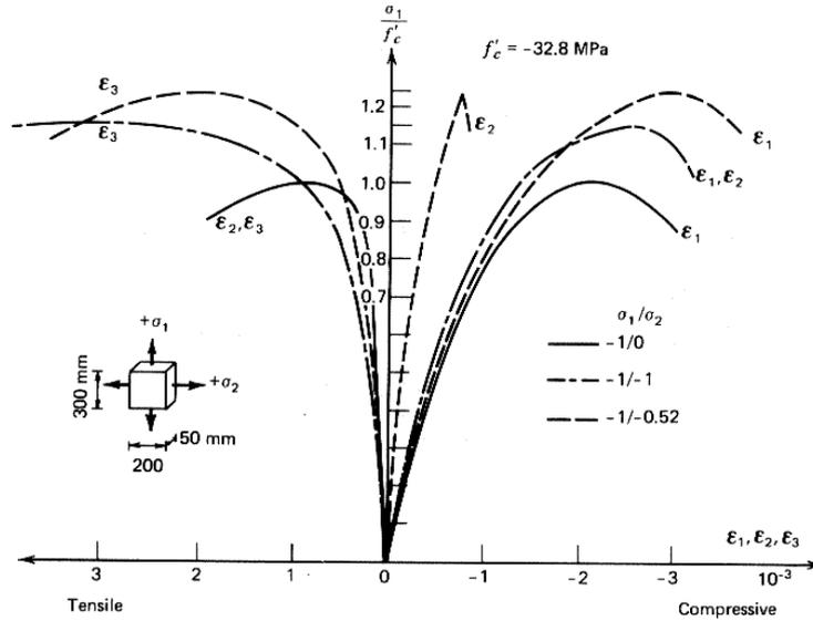
**Fig.2 stress-strain relationships of concrete under biaxial compression test [9]**
