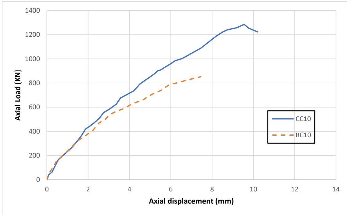
**Fig.11(a) Load – Axial displacement relationship of CC10 and RC10**
