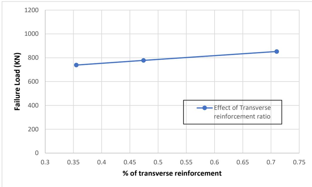
**Fig.8 Effect of Transverse Reinforcement Ratio on Failure load**
