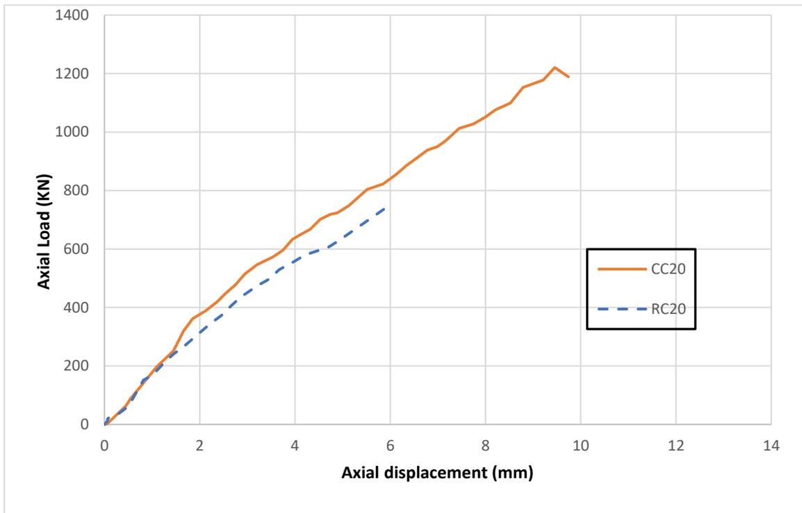
**Fig.11(b) Load – Axial displacement relationship of CC20 and RC20**
