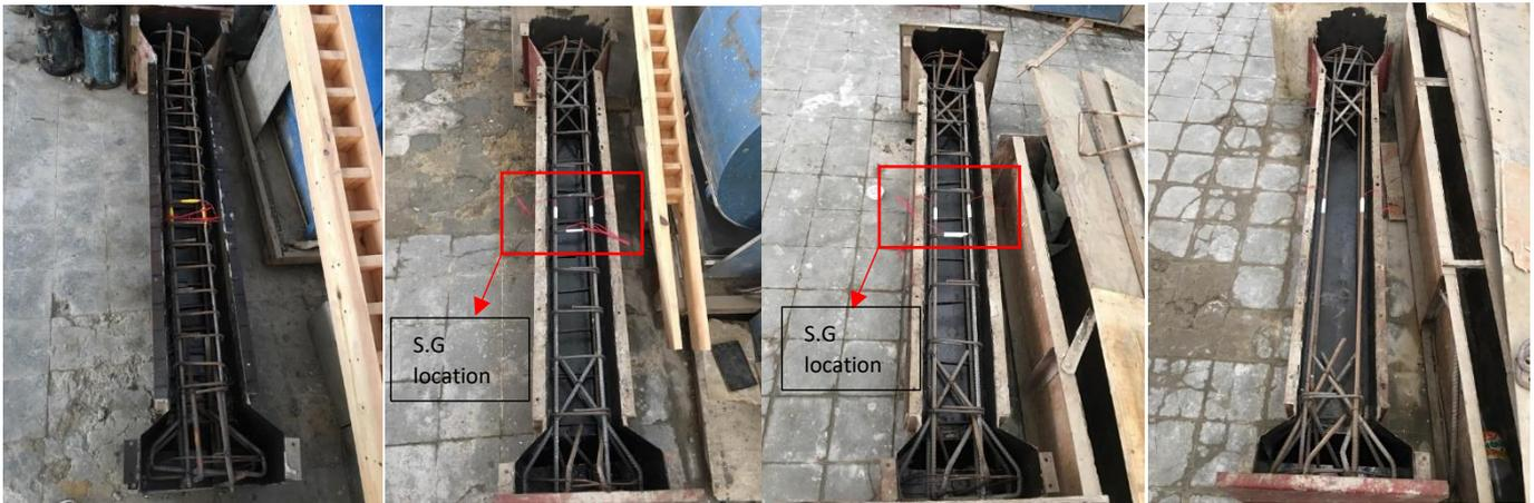
**Fig.3 Reinforcement arrangement of columns specimens in the steel formwork**
