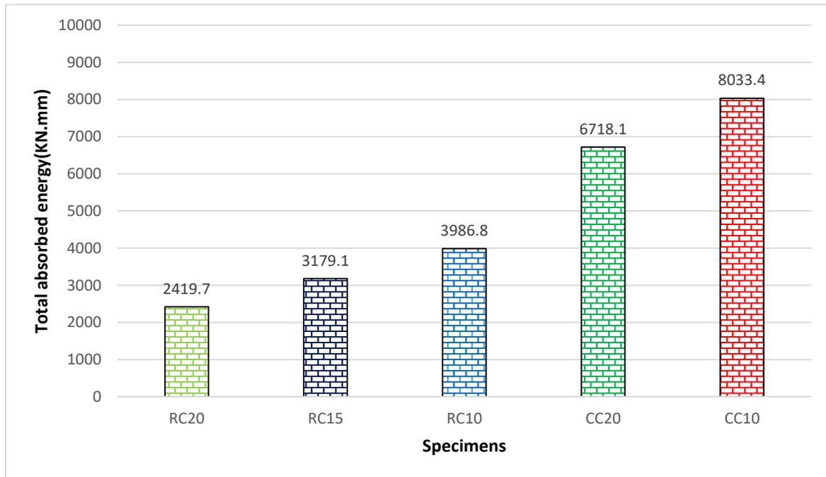
**Fig.12 Total absorbed energy of specimens**
