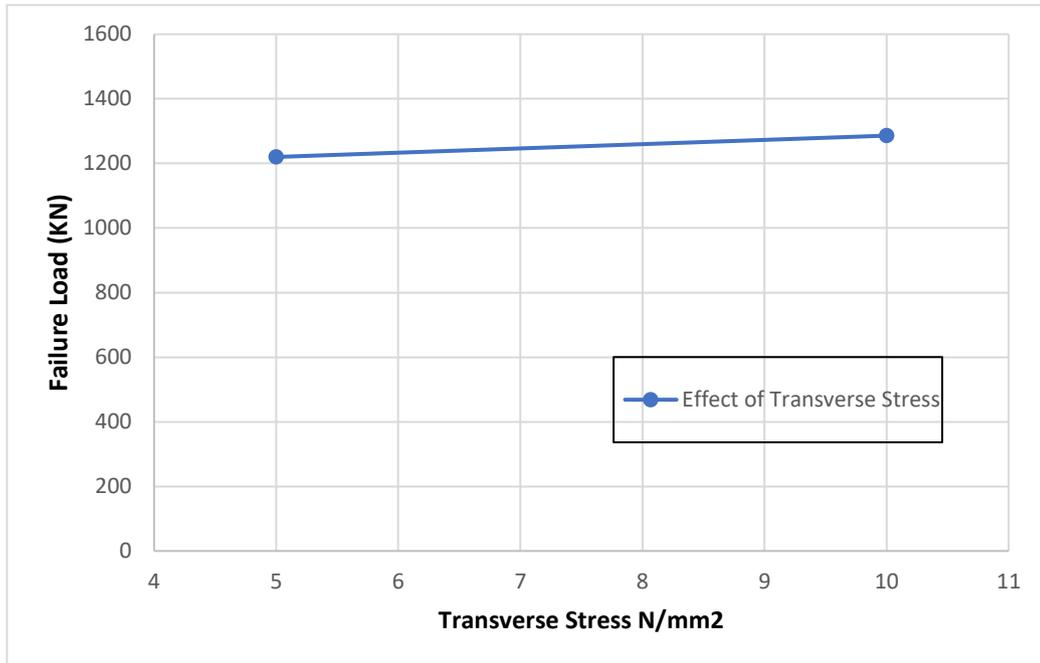
**Fig.10 Effect of Transverse Stress on Failure load**
