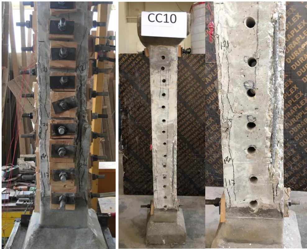
**Fig.6 (b). Crack Patterns for Specimen CC10**
