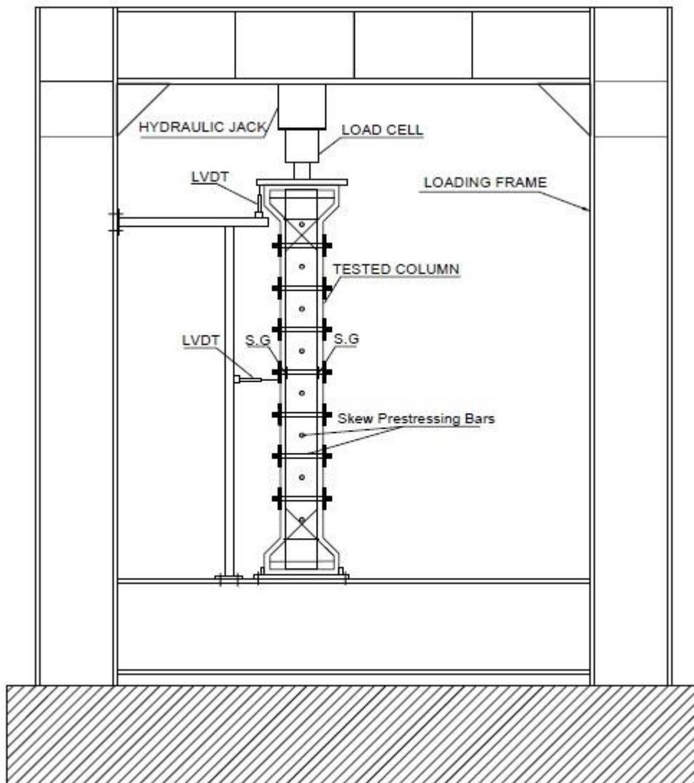
**Fig.5 Schematic Diagram for Testing Frames and Test Setup**
