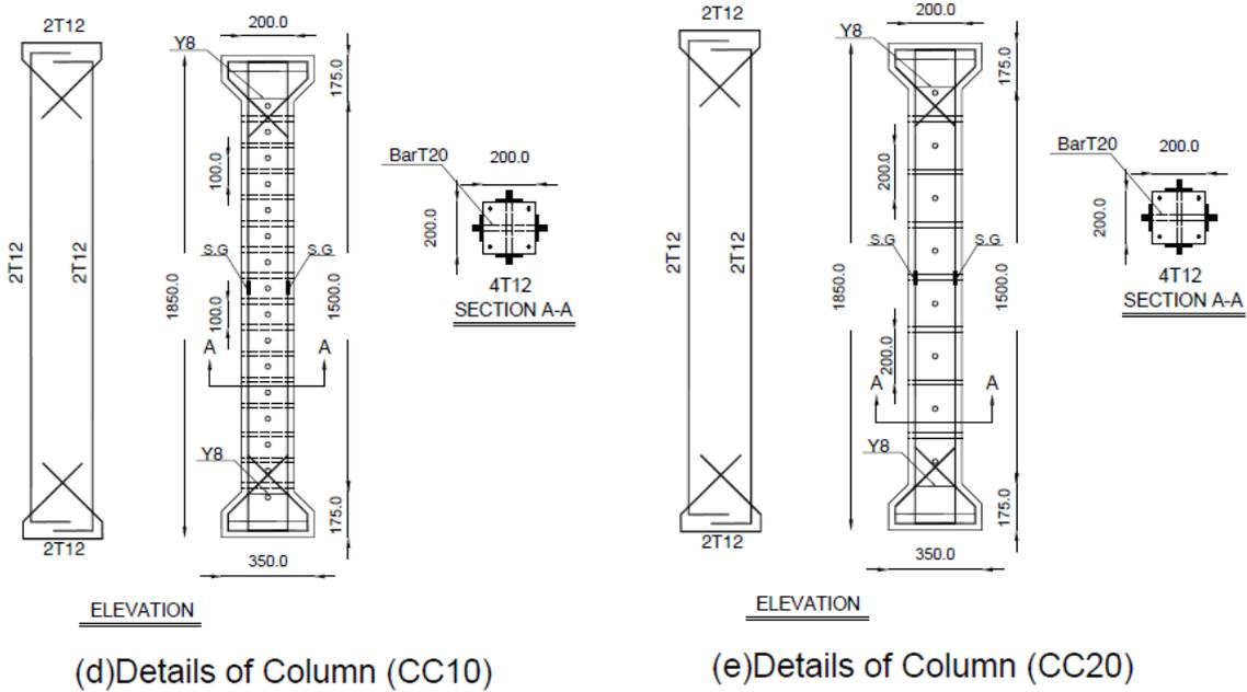
**Fig.4 Details of Tested Columns**
