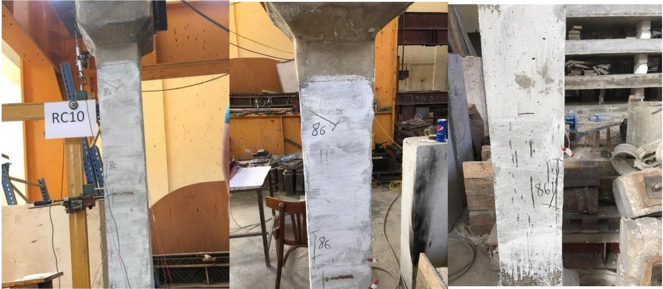
**RC10****Fig.6 (c). Crack Patterns for Specimen (RC20, RC15and RC10)****Table (3): The Experimental Results of the Tested Columns.**
