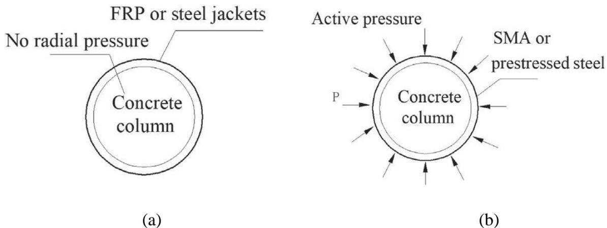
**Fig.1 (a) passive and (b) active confinement on concrete column cross-sections [1].**
