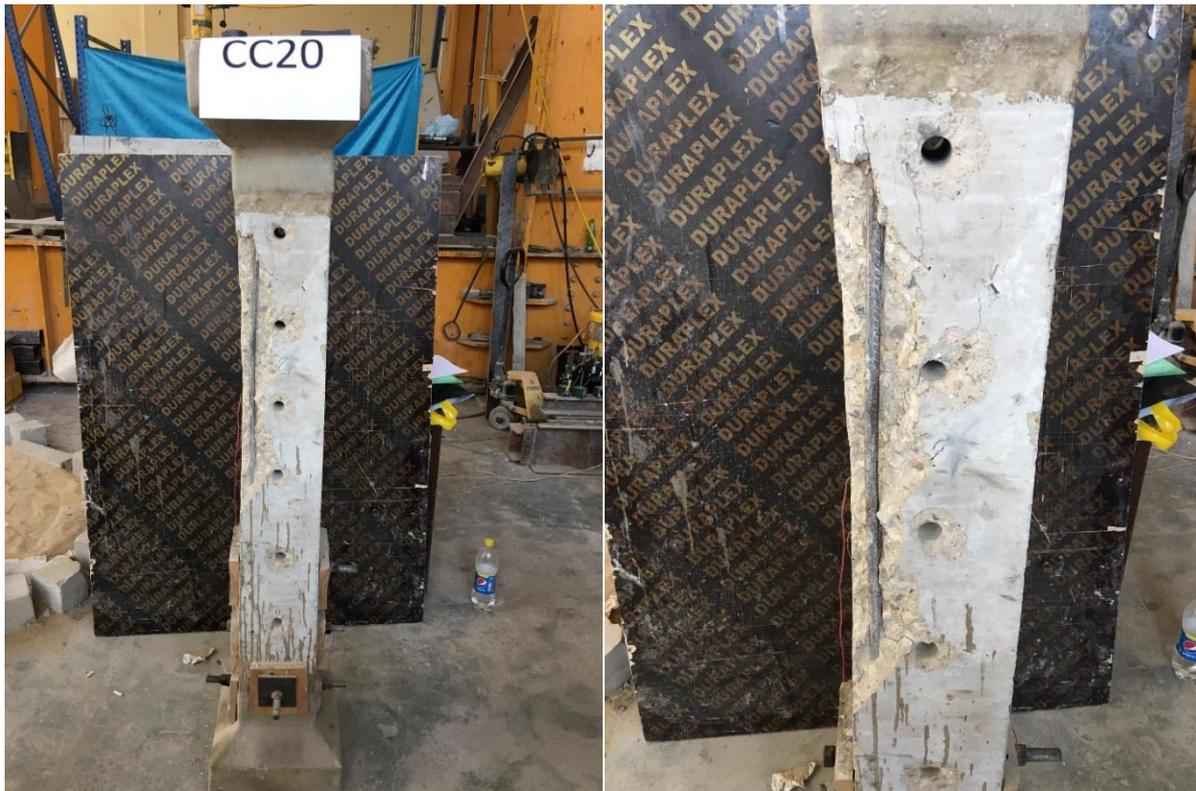
Fig.6 (a). Crack Patterns for Specimen CC20
