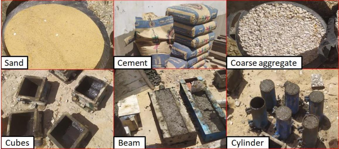
Figure (2): Materials, Samples preparation in laboratory
