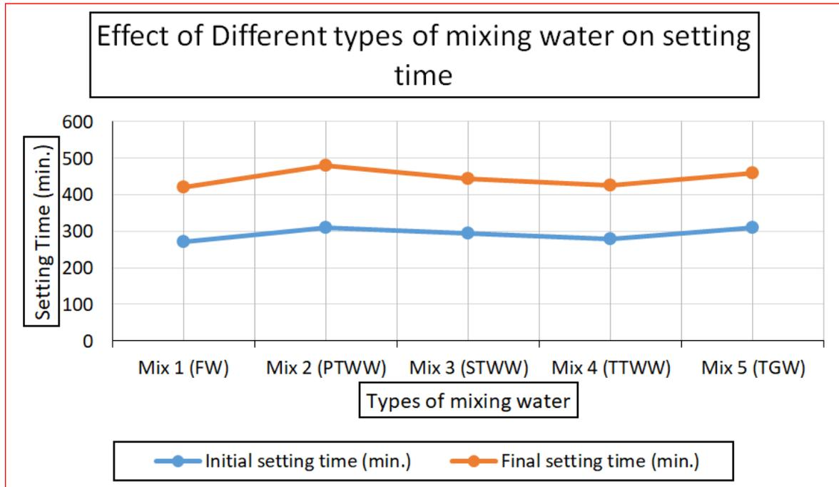
**Figure (7): Effect of Different types of mixing water on setting time**
