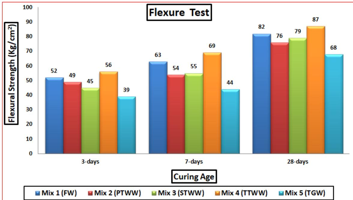
**Figure (6): Influence of different types of Treated wastewater on Concrete bending moment at various curing age**
