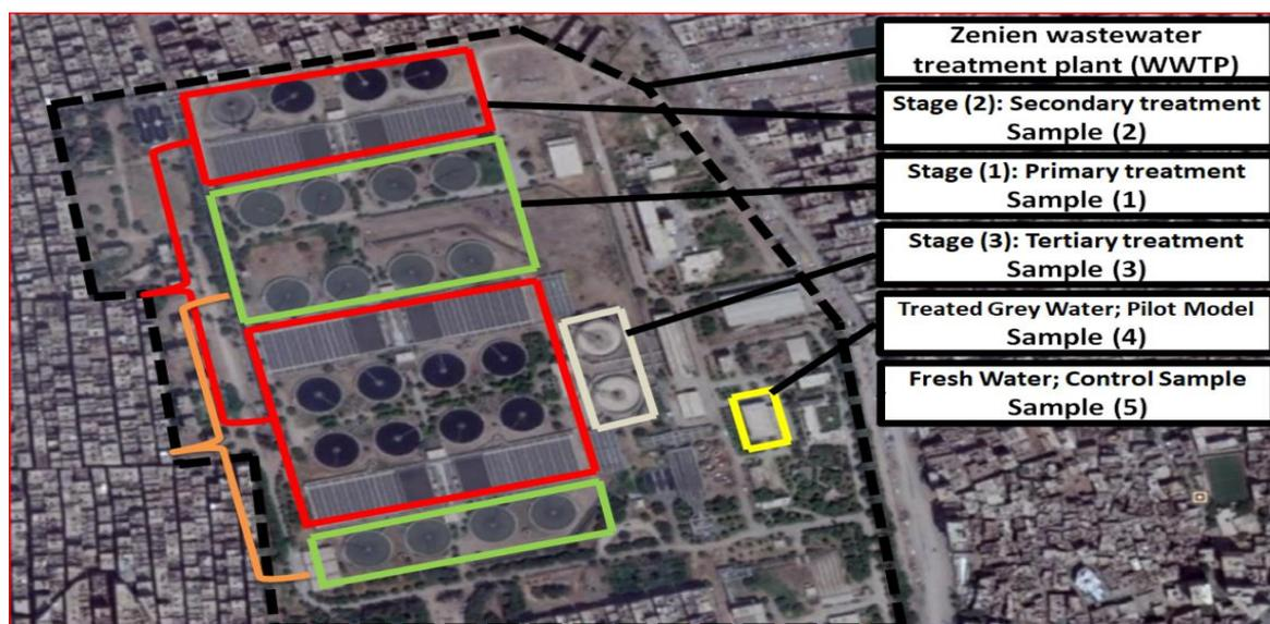
Figure (1): Stages of Zenien wastewater treatment plant (WWTP)
