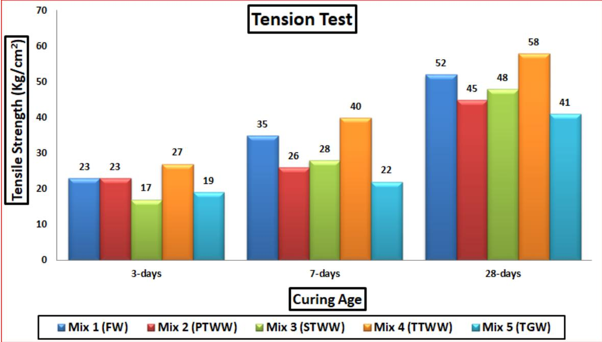
Figure (5): Influence of different types of Treated wastewater on Concrete tensile strength at various curing age
