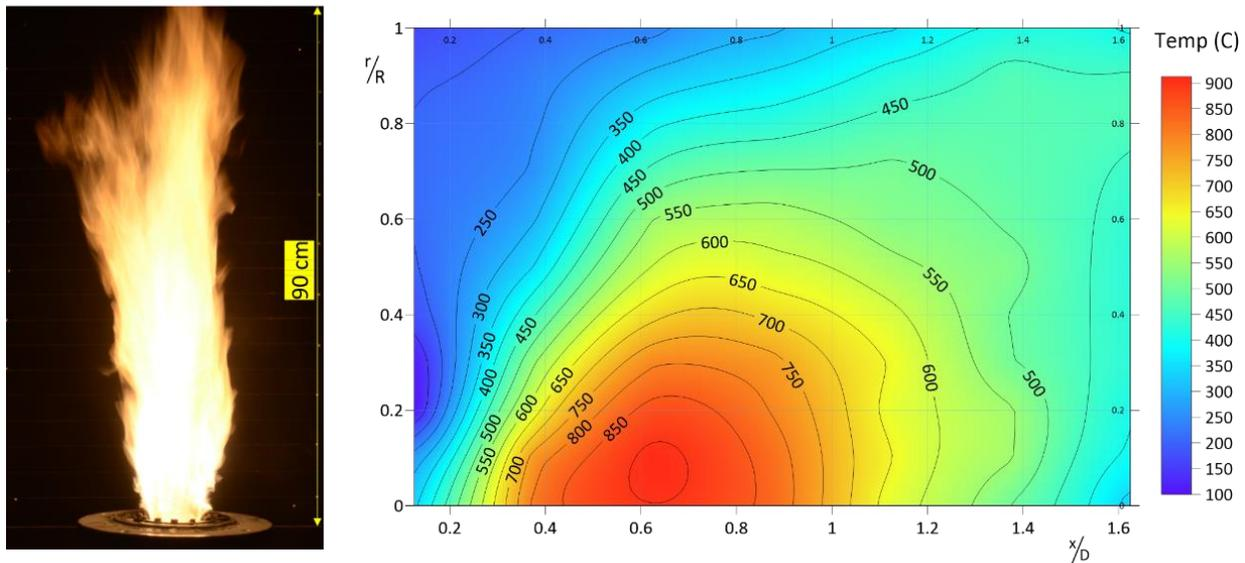
**Figure 4 photograph of vertical oil firing (Left), Temperature contours inside the furnace (Right), Run 1**
