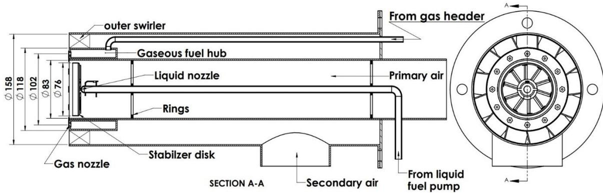
Panel (b) Design details of Burner
