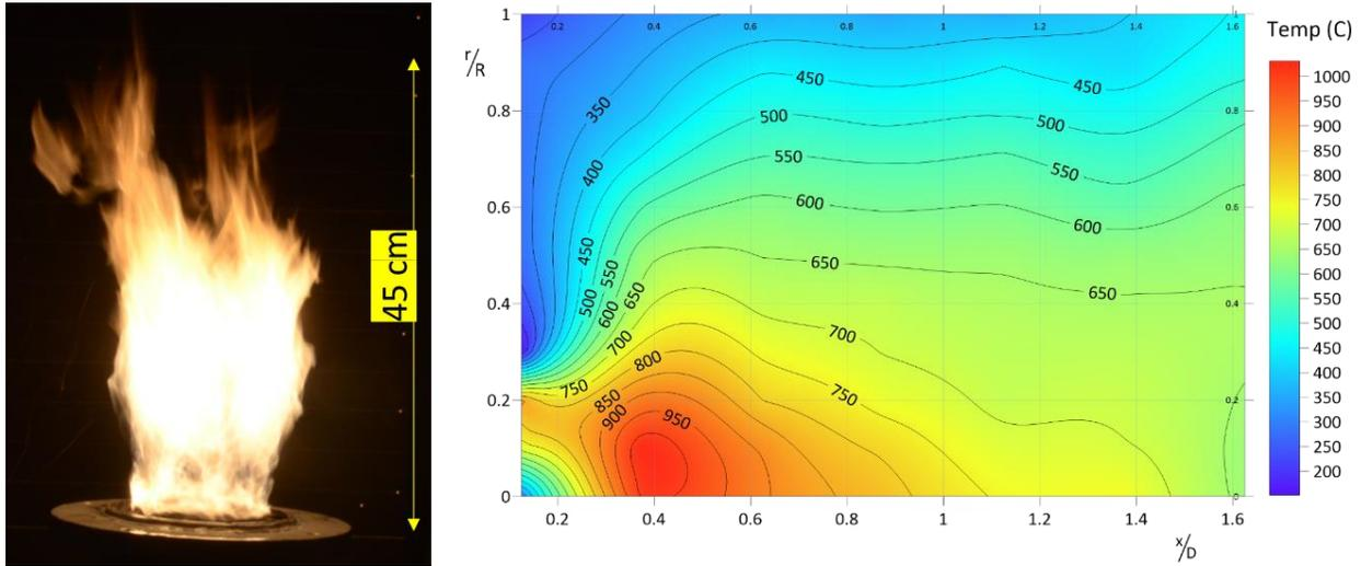
Figure 6 photograph of vertical cofiring of LPG and Light diesel fuels (Left), Temperature contours inside the furnace (Right), Run 3
