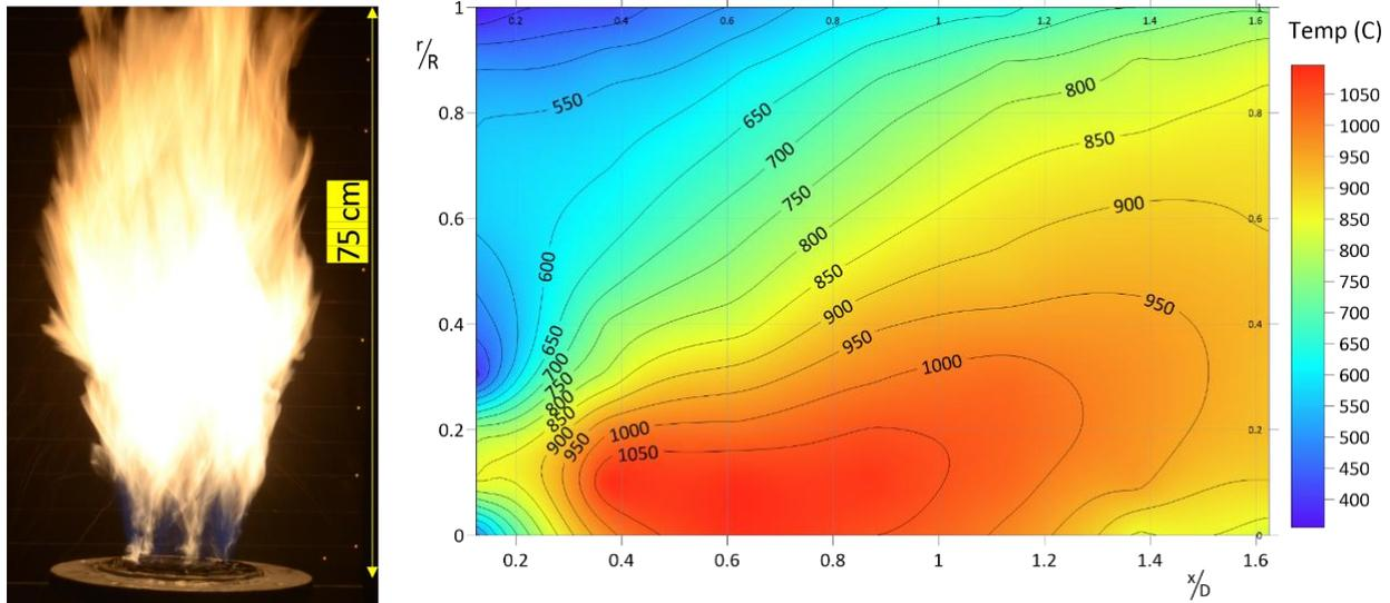
**Figure 5** photograph of vertical gas firing (Left), Temperature contours inside the furnace (Right), Run 2
