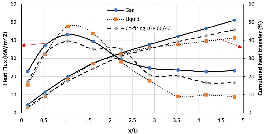
Figure 7 Comparison of heat flux on the furnace wall and cumulated heat transferred to cooling water jacket
