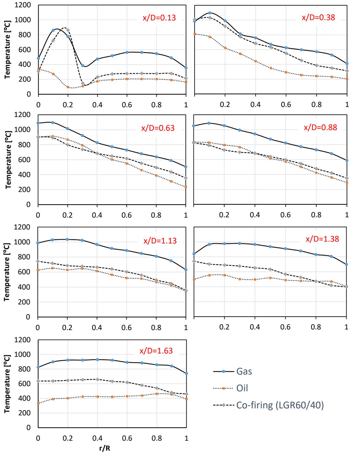
Figure 8 Radial temperature distributions at each measuring hole ( $x/D$ )
