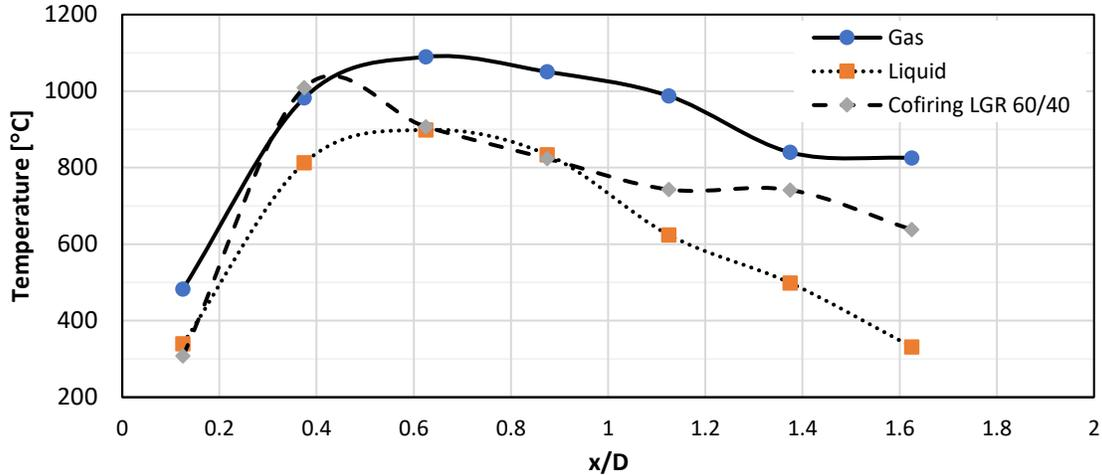
**Figure 9 Axial temperature distribution along the centerline of the furnace**
