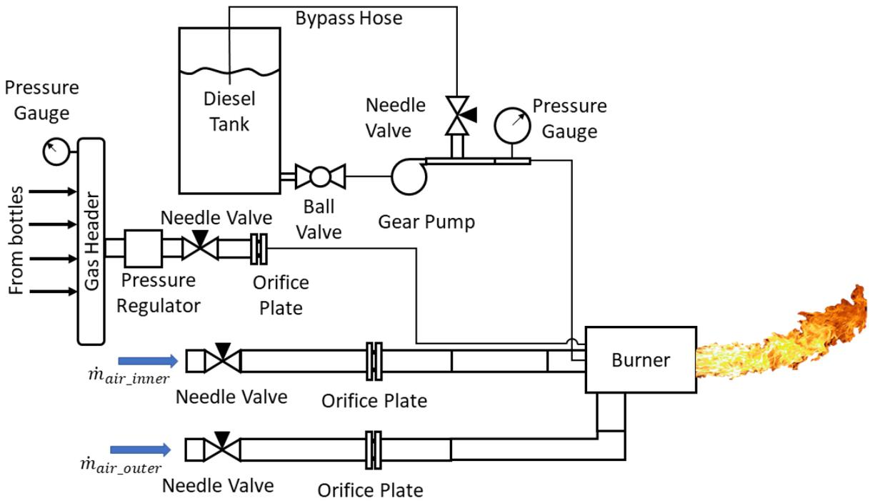
Figure 2 The gaseous and oil fuel feeding lines
