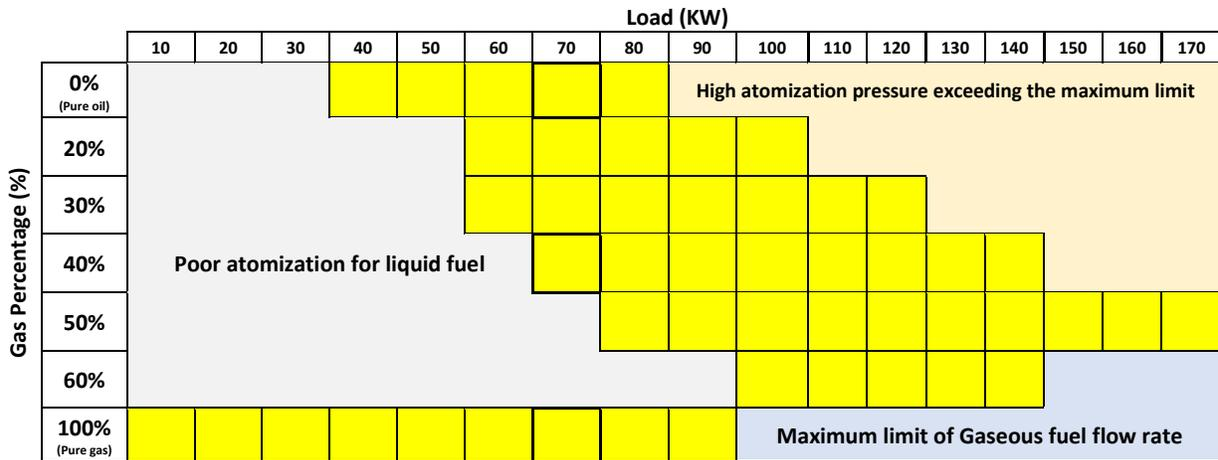
This load mapping suggests using an air-assisted atomizer instead of the pressure jet atomizer to unlink the thermal load from the quality of atomization, which expands the available region of operation and ensures better atomization for cofiring cases.
