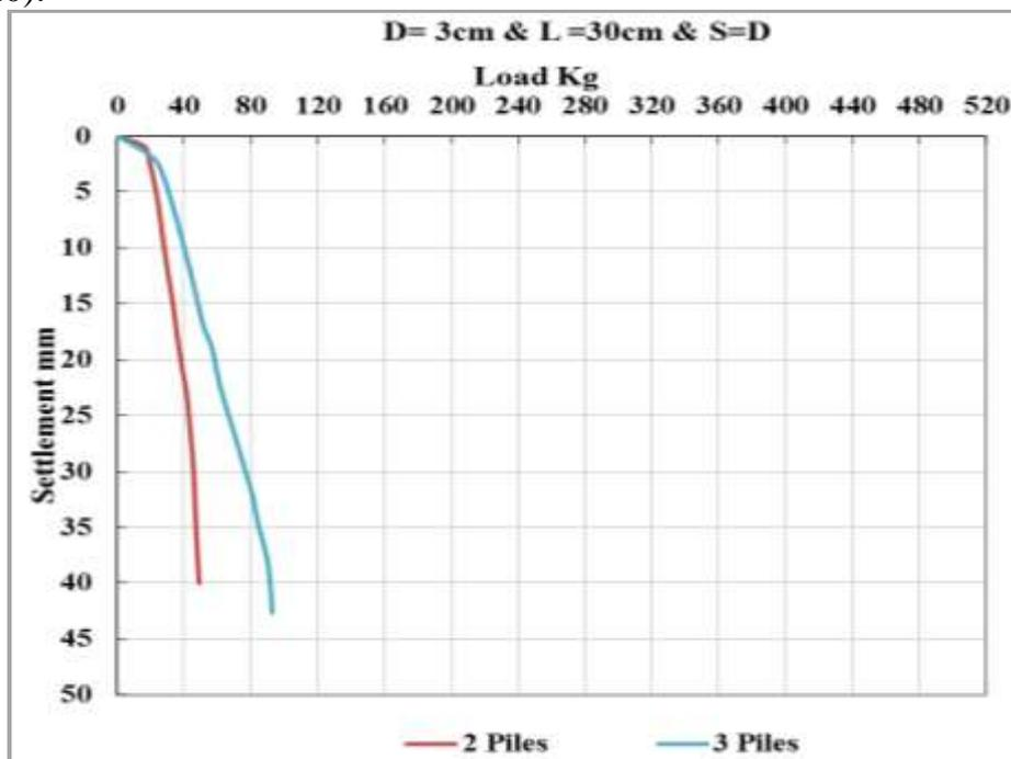
**Fig. (6): Load –Settlement curve for (2 x1) and (3 x1) pile group with spacing (S =D)**
