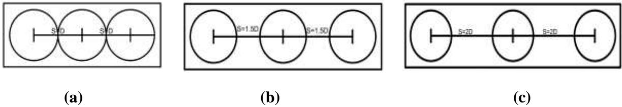
**Fig. (4) : Pile group arrangements for 3 Piles with spacing between piles**
