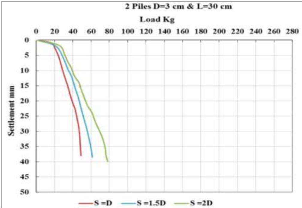
Fig. (9): Load –Settlement curve for (2 x 1) pile group with spacing (S = D,1.5D and 2D)
