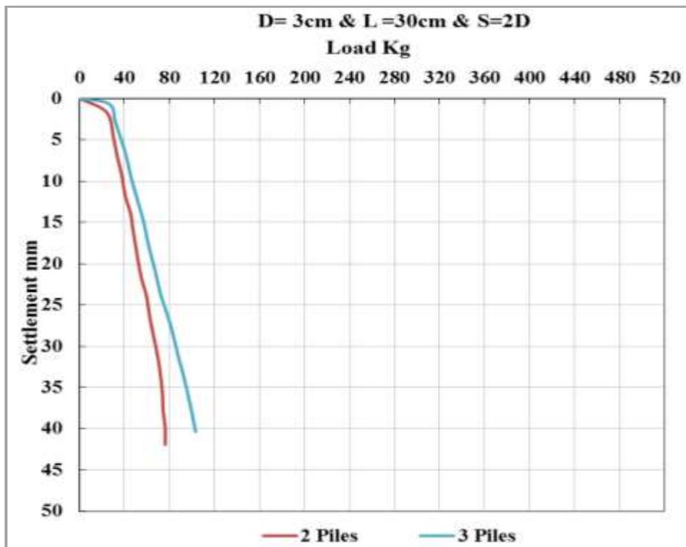
Fig. (8): Load –Settlement curve for (2x1) and (3x1) pile group with spacing (S = 2D)
