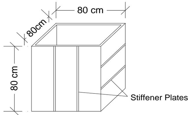
**Fig. (5): Details of Steel tank used in model test**
