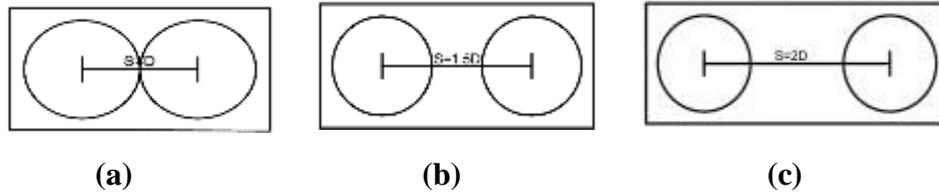
**Fig. (3) : Pile group arrangements for 2 Piles with spacing between piles**
