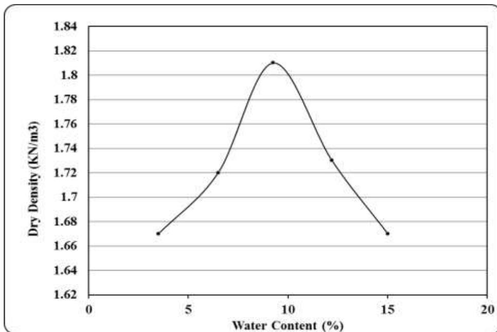
**Fig. (2): Compaction characteristics of the used Sand**
