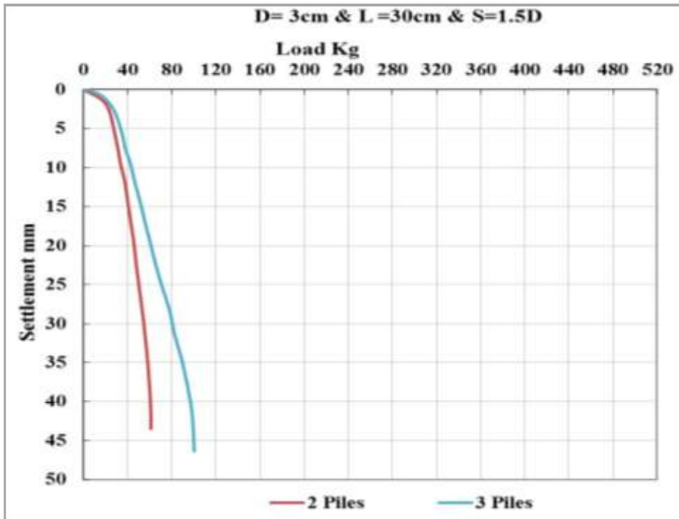
Fig. (7): Load –Settlement curve for (2 x 1) and (3 x 1) pile group with spacing (S=1.5D)
