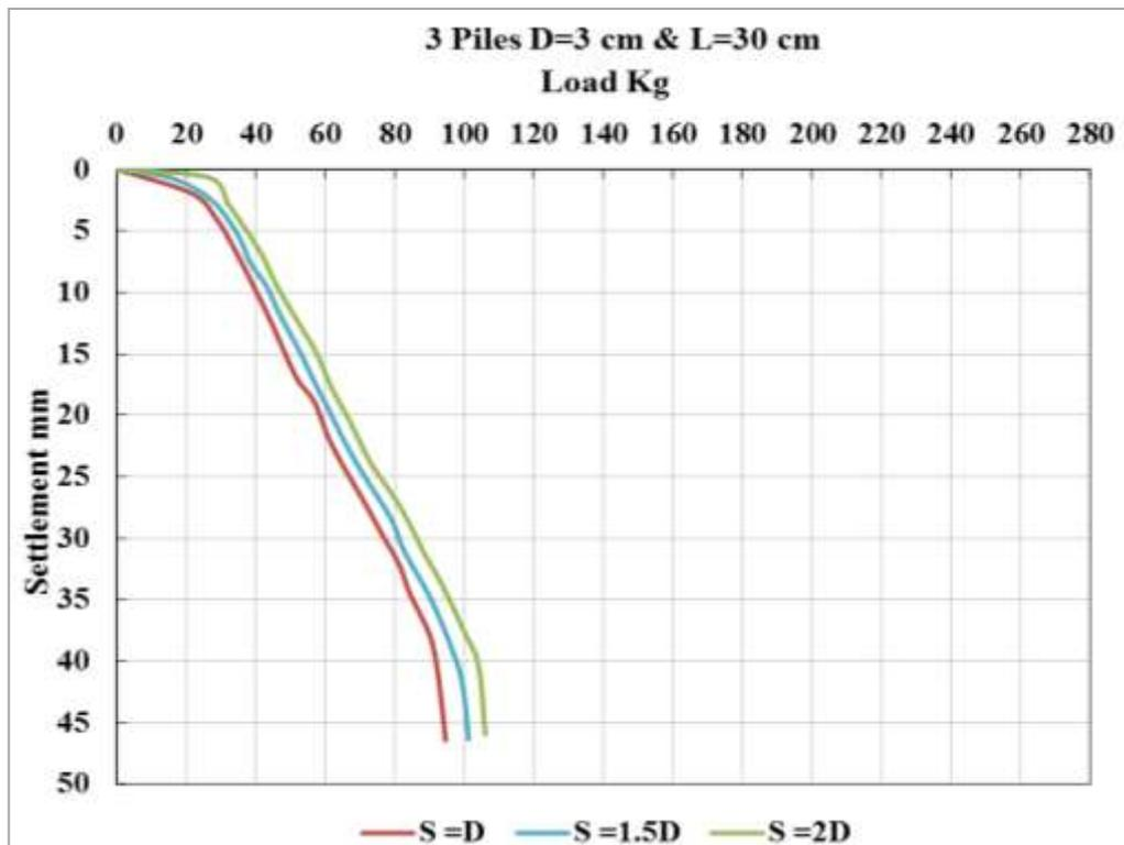
Fig. (10): Load –Settlement curve for (3x1) pile group with spacing (S= D,1.5D and 2D)
