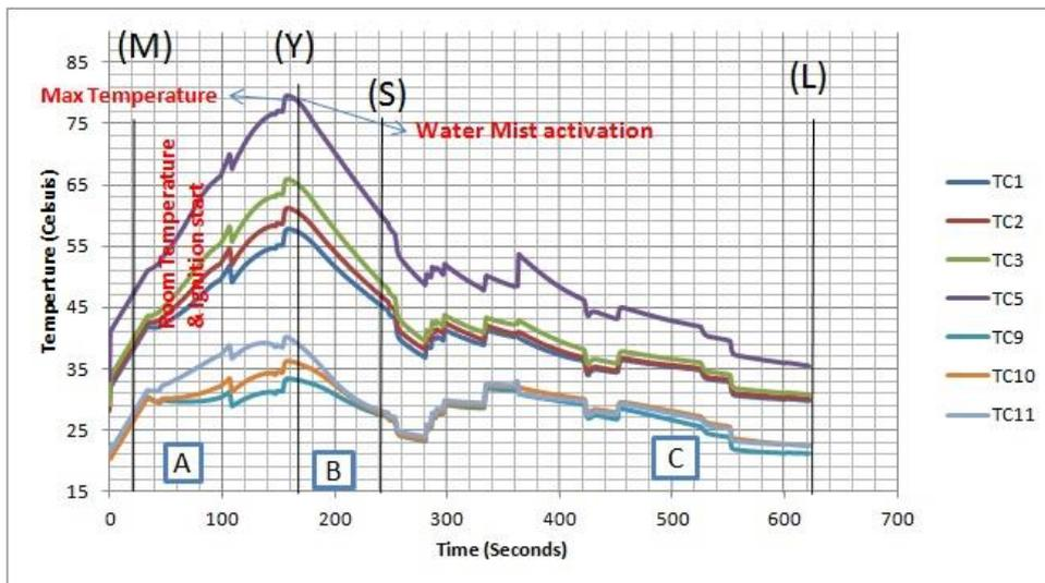
Figure 8 Fire Test With LPWM Nozzle (Tyco AM27)
