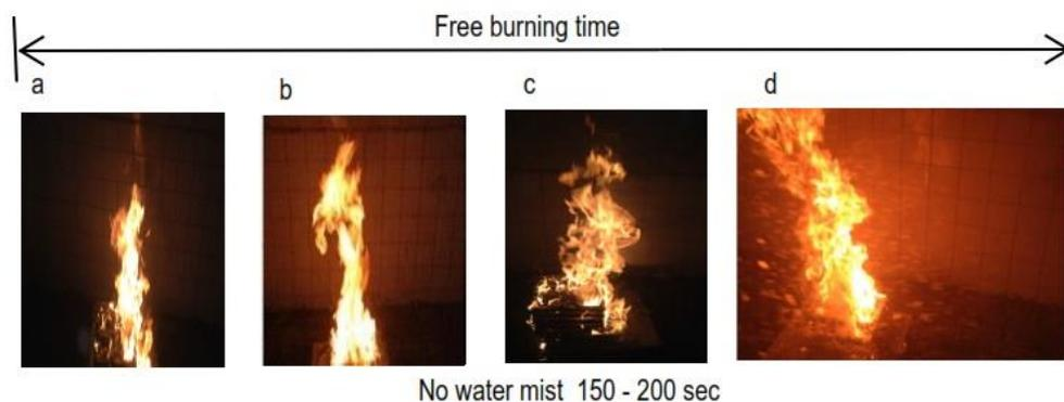
**Figure 2 Free Burning period for PMMA fires Before water mist discharged fixed for all fire tests.**
