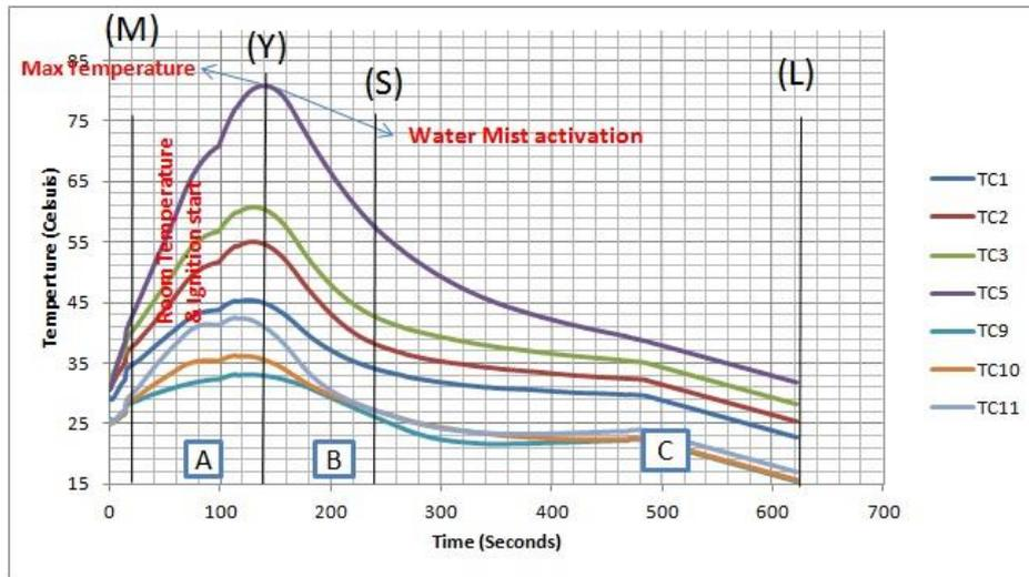
**Figure 9 Fire Test with Conventional Nozzle (Viking)**
