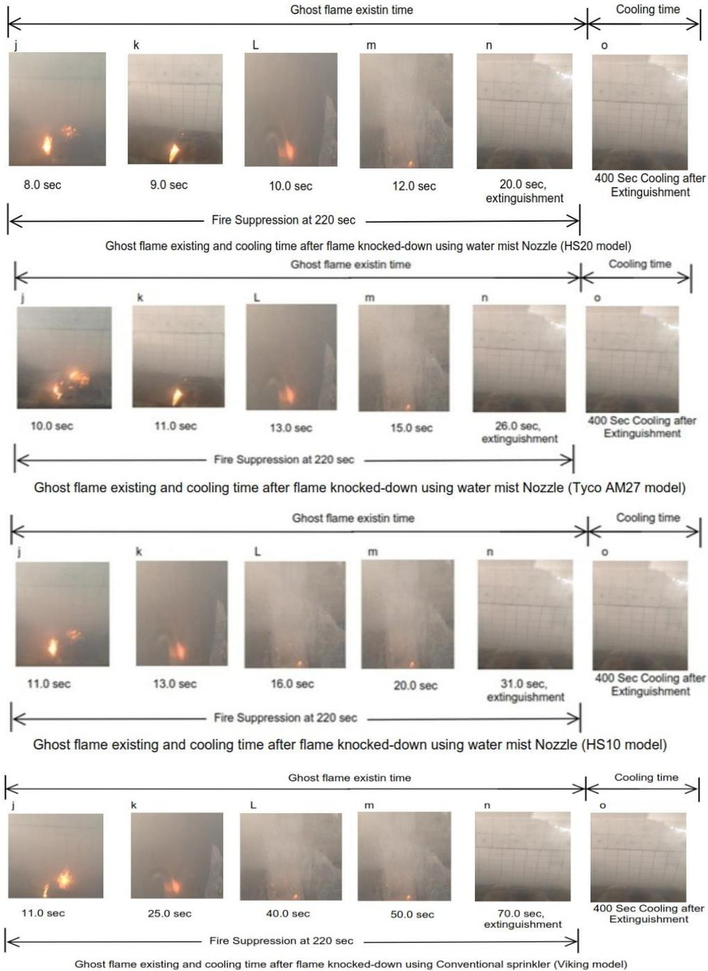
**Fig.4 Ghost flame existing and cooling time after flame knocked-down**
