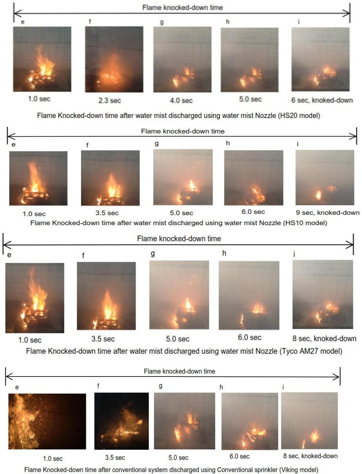
**Fig.3 Flame Knocked-down time after water mist discharged**
