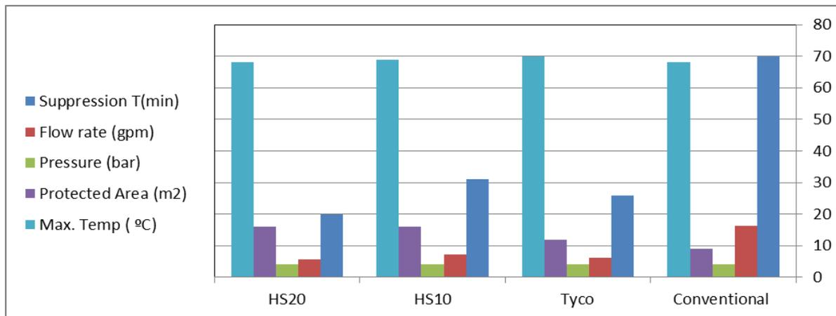
**Figure 10 Comparison between fire test results.**
