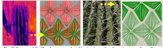
Fig. (8).Set up model in Grasshopper to evaluate biomimetic envelope for saving energy for cooling. Source: by Researcher.
