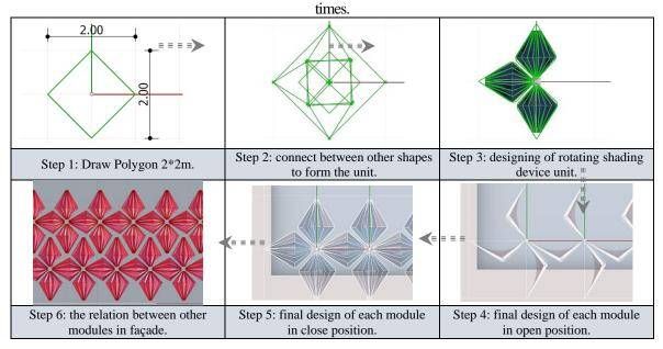
The shading device systems contain stainless steel supporting frames, aluminum dynamic frames, and fiberglass mesh infill. The rotating system transforms the shading screen from a seamless veil into a lattice-like pattern to provide shade or light. Each shading device comprises a series of stretched (PTFE) panels.
