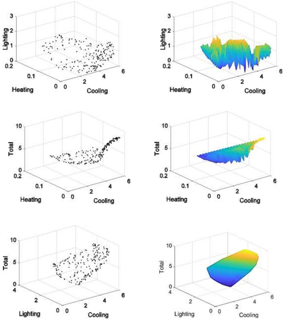
Figure (11) Pareto fronts of the triple-objective optimization
