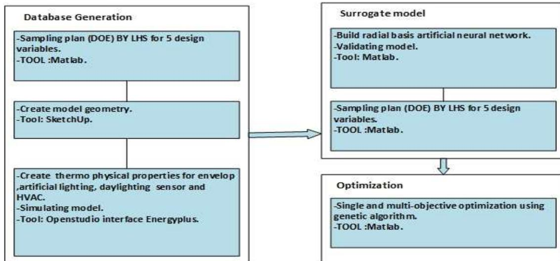
Figure (4): A flowchart of the surrogate-based optimization approach
