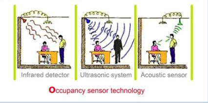
Figure 6: Occupancy sensor technology (www.iklimnet.com)
