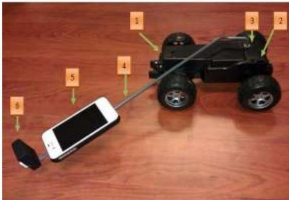
Fig.2, [3]:Truck platform structure design. (1) The stepper motor for steering the front two wheels, (2) The back motor to control the back wheels, (3) The third motor to rotate the fiber arm in a circular shape with 50cm radius to increase the scanned area,(4) The fiber arm with 50cm length, (5) The smart cellphone that act as a metal detector sensor, (6)The GSM Audio\Sound tracker and GPS sensors.
