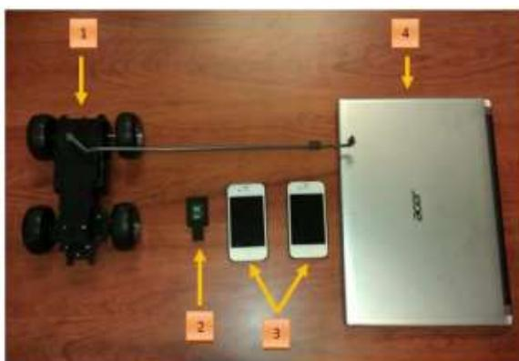
Fig.1,[3]: Hardware component for the proposed solution.(1) RC truck with a movable fiber arm, (2) Mini GPS + GSM audio\sound tracker + SIM card, (3)Two smart cellular based on Android OS, (4)Laptop equipped for wireless connectivity to the internet in addition to the spatial database.
