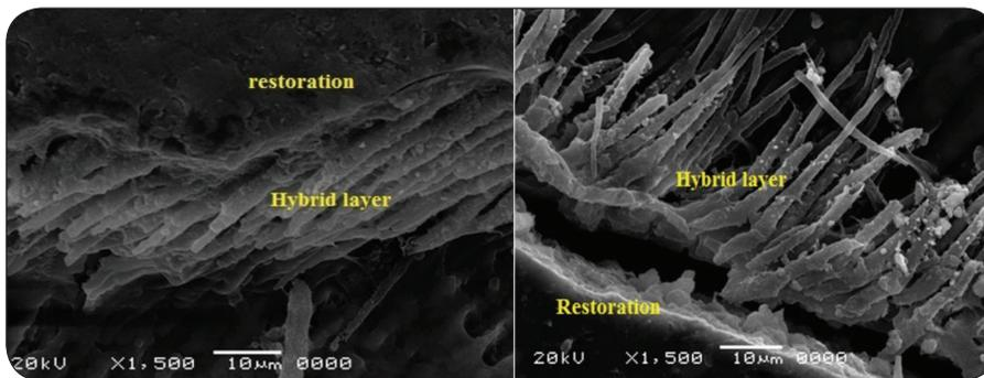
Fig. (3) Scanning electron photomicrograph for the resin dentin interface (at 1500X) of Sonic fill at 6 months storage showing gap at the interface (left) and for the resin dentin interface (at 1500X) of Ceram X at six months storage showing gap at the interface (right).
